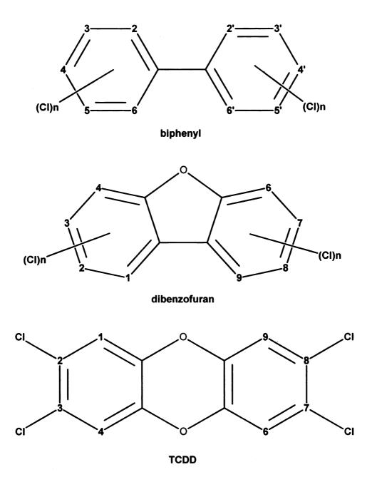
Figure 1.2. Chemical structure of 2,3,7,8-tetrachlorodibenzo-p-dioxin (TCDD), and general dibenzofuran and biphenyl rings with potential halogenation sites numbered.
