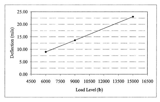
Figure C-8 Deflection Data vs. Load Level Linearity Plot for Site #9
