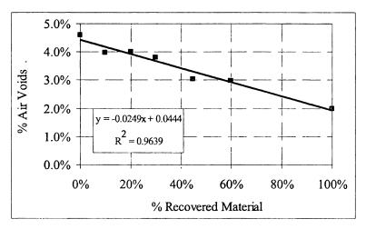
Figure 4.17 Air voids versus percent recovered material for a wearing course recycled mixture with Deena aggregates and Mandra recovered material (Superpave Mixture)
