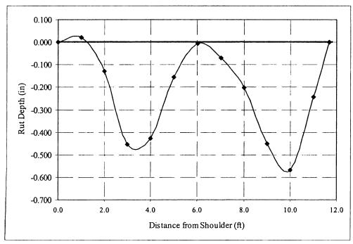
Figure B-32 Average profile of test site 7
