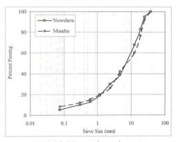
Figure 3.12 Gradation curve of recovered aggregates
