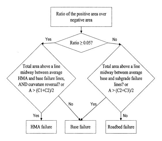
Figure 4.2 Conditions for determining the rutting seat (NCHRP 2002)
