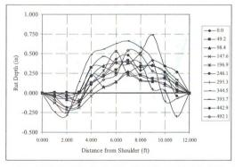
Figure B-16 Horizontal profiles from 0 - 492.1 ft along test site 6, section 3
