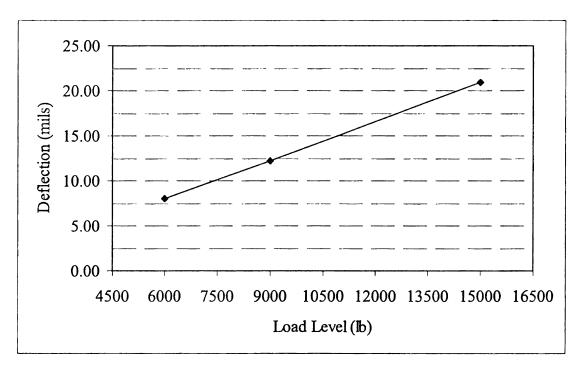
Figure C-4 Deflection Data vs. Load Level Linearity Plot for Site #5
