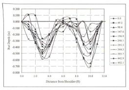
Figure B-19 Horizontal profiles from 0 - 492.1 ft along test site 7, section 3
