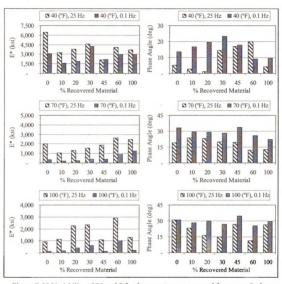
Figure E-28 Variability of E\* and  $\delta$  for the same temperature and frequency for base course Deena + Mandra blends
