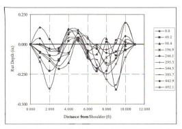
Figure B-1 Horizontal profiles from 0 - 492.1 ft along test site 1, section 1
