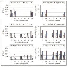
Figure E-22 Variability of E\* and  $\delta$  for the same temperature and frequency for wearing course Margalla + Mandra blends
