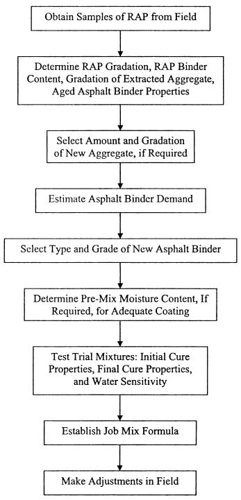
Figure 2.18 Flow chart for mix design of cold recycled mixes
