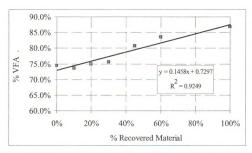
Figure 4.19 VFA versus percent recovered material for a wearing course recycled mixture with Margalla aggregates and Mandra recovered material (Superpave Mixture)
