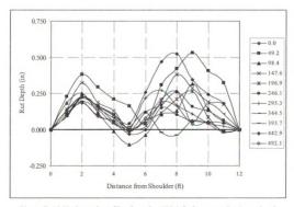
Figure B-10 Horizontal profiles from 0 - 492.1 ft along test site 4, section 3
