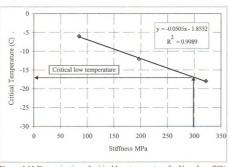
Figure 4.11 Determination of critical low temperature for Nowshera 70%
