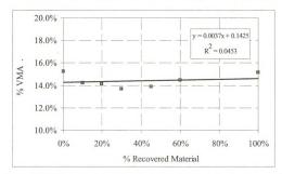
Figure 4.18 VMA versus percent recovered material for a wearing course recycled mixture with Deena aggregates and Mandra recovered material (Superpave Mixture)
