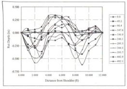
Figure B-11 Horizontal profiles from 0 - 492.1 ft along test site 5, section 1
