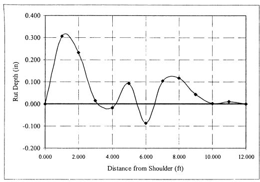
Figure B-33 Average profile of test site 8
