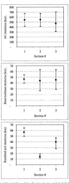
Figure C-14 Variability of the Backcalculated Moduli for Site #3
