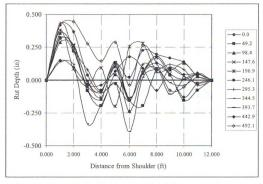
Figure B-20 Horizontal profiles from 0 - 492.1 ft along test site 8, section 1
