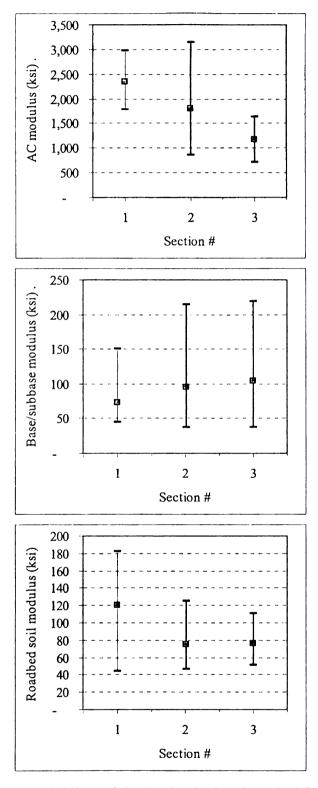
Figure C-23 Variability of the Backcalculated Moduli for Site #12
