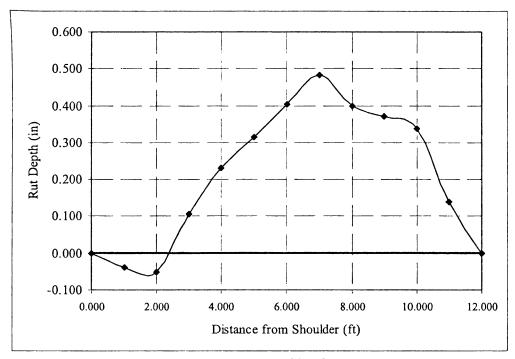
Figure B-31 Average profile of test site 6
