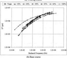
Figure 4.24 Master curve for the Margalla + Mandra recycled mixtures
