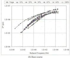
Figure 4.26 Master curve for the Deena + Mandra recycled mixtures
