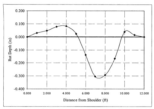
Figure B-27 Average profile of test site 2
