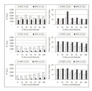
Figure 4.21 Variability of  $E^*$  and  $\delta$  for the same temperature and frequency for wearing course Margalla + Nowshera (MW-N) blends
