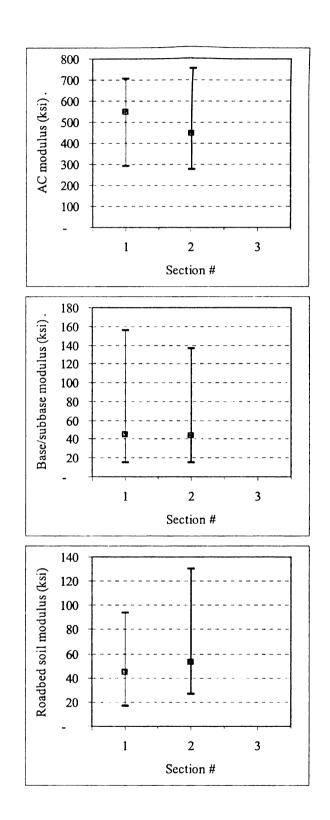
Figure C-21 Variability of the Backcalculated Moduli for Site #10
