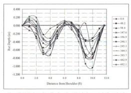
Figure B-18 Horizontal profiles from 0 - 492.1 ft along test site 7, section 2
