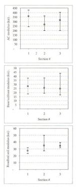
Figure C-15 Variability of the Backcalculated Moduli for Site #4
