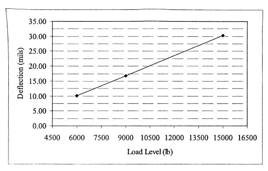
Figure C-7 Deflection Data vs. Load Level Linearity Plot for Site #8
