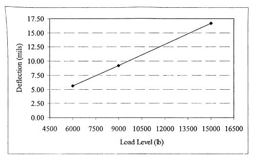
Figure C-9 Deflection Data vs. Load Level Linearity Plot for Site 10
