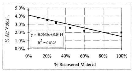
Figure E-11 Air voids versus percent recovered material for DB-M (Superpave Mixture)
