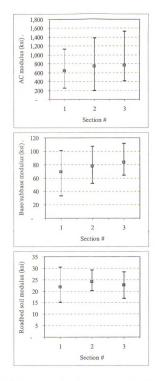
Figure C-18 Variability of the Backcalculated Moduli for Site #7
