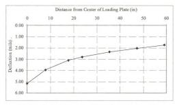
Figure 4.6 Deflection basin of sensors D0, D1 and D3 through D7
