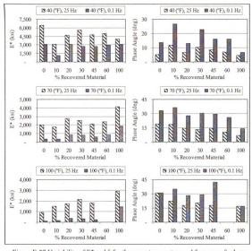
Figure E-27 Variability of E\* and  $\delta$  for the same temperature and frequency for base course Deena + Nowshera blends
