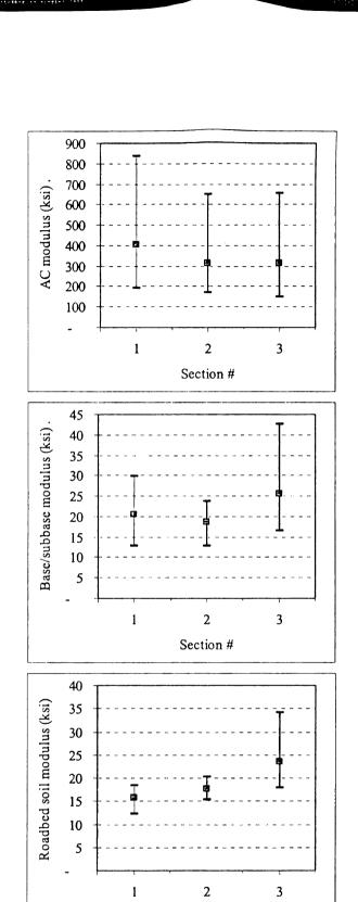
Figure C-17 Variability of the Backcalculated Moduli for Site #6
