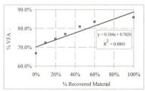
Figure E-18 VFA versus percent recovered material for DB-M (Superpave Mixture)
