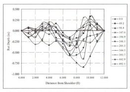
Figure B-4 Horizontal profiles from 0 - 492.1 ft along test site 2, section 1
