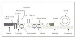
Figure 2.6 Concept of remixing method
