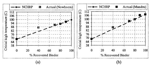
Figure 4.14 Critical high temperatures versus predicted for Nowshera blends (a) and Mandra blends (b)
