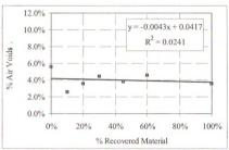
Figure E-1 Air voids versus percent recovered material for a wearing course recycled mixture with Deena aggregates and Nowshera recovered material (Marshall Mixture)
