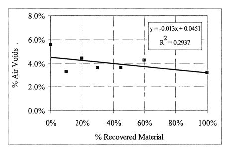
Figure 4.16 Air voids versus percent recovered material for a wearing course recycled mixture with Deena aggregates and Mandra recovered material (Marshall Mixture)
