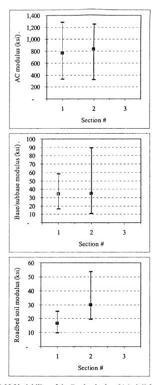
Figure C-22 Variability of the Backcalculated Moduli for Site #11
