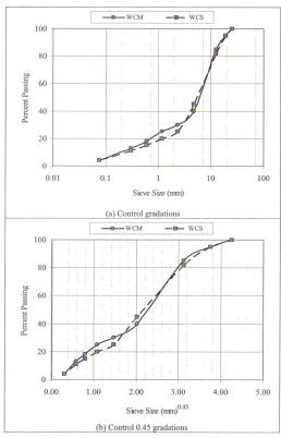
Figure 3.10 Wearing course control gradations (Marshal and Superpave) – 19 mm nominal maximum aggregate size
