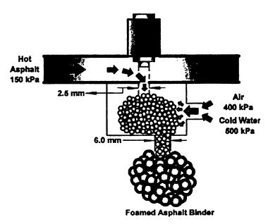
Figure 2.12 Process of asphalt foaming (Kim, 2006)
