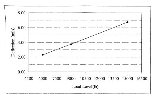
Figure C-11 Deflection Data vs. Load Level Linearity Plot for Site #12
