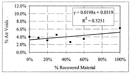
Figure E-7 Air voids versus percent recovered material for a base course recycled mixture with Margalla aggregates and Nowshera recovered material (Marshall Mixture)
