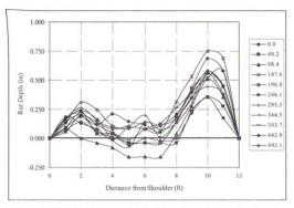
Figure B-9 Horizontal profiles from 0 – 492.1 ft along test site 4, section 2
