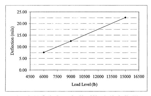
Figure C-10 Deflection Data vs. Load Level Linearity Plot for Site #11
