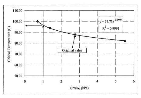
Figure 4.10 Determination of critical high temperature for Mandra 70%
