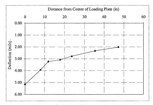
Figure 4.5 Deflection basin of sensors D0 through D6
