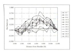
Figure B-15 Horizontal profiles from 0-492.1 ft along test site 6, section 2
