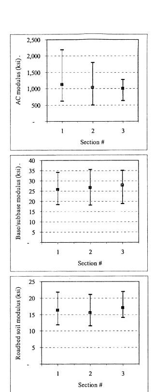
Figure C-16 Variability of the Backcalculated Moduli for Site #5
