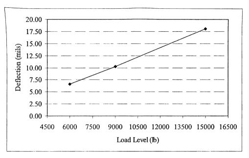
Figure C-5 Deflection Data vs. Load Level Linearity Plot for Site #6
