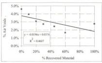
Figure E-8 Air voids versus percent recovered material for DW-N (Superpave Mixture)
