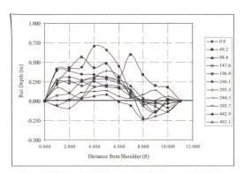
Figure B-3 Horizontal profiles from 0 - 492.1 ft along test site 1, section 3
