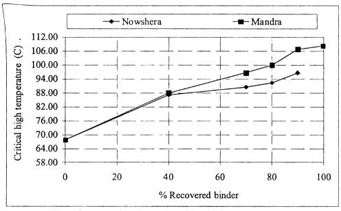
Figure 4.12 Effect of recovered binder on the critical high temperature for Nowshera and Mandra
