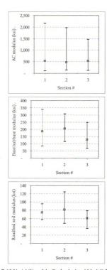
Figure C-13 Variability of the Backcalculated Moduli for Site #2
