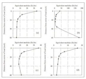
Figure 4.7 Plots used in determining the presence of a stiff layer
