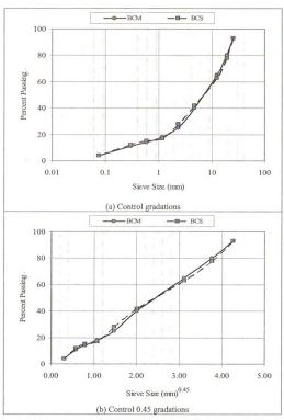
Figure 3.11 Base course control gradations (Marshal and Superpave) – 25 mm nominal maximum aggregate size
