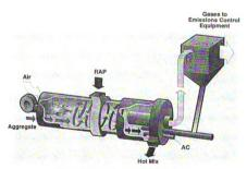
Figure 2.2 RAP in a parallel flow drum
