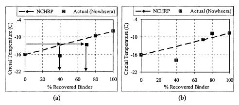
Figure 4.15 Critical low temperatures versus predicted for Nowshera blends (a) and Mandra blends (b)
