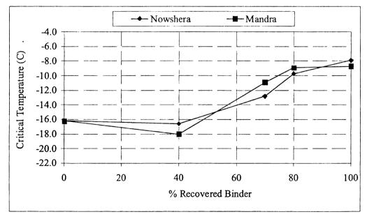
Figure 4.13 Effect of recovered binder on the critical low temperature for Nowshera and Mandra
