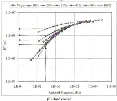
Figure 4.23 Master curve for the Margalla + Nowshera recycled mixtures
