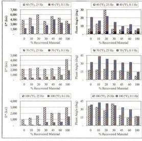
Figure E-25 Variability of E\* and  $\delta$  for the same temperature and frequency for base course Margalla + Nowshera blends
