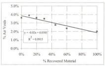
Figure E-9 Air voids versus percent recovered material for MW-N (Superpave Mixture)
