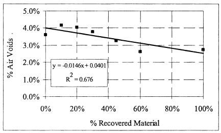
Figure E-10 Air voids versus percent recovered material for MW-M (Superpave Mixture)
