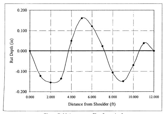
Figure B-30 Average profile of test site 5
