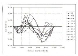
Figure B-7 Horizontal profiles from 0 - 492.1 ft along test site 3, section 1
