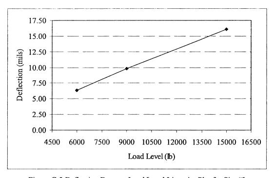
Figure C-2 Deflection Data vs. Load Level Linearity Plot for Site #3
