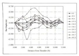
Figure B-13 Horizontal profiles from 0 - 492.1 ft along test site 5, section 3
