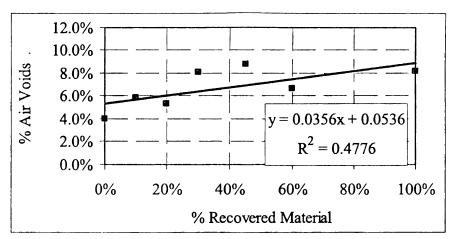
Figure E-6 Air voids versus percent recovered material for a base course recycled mixture with Margalla aggregates and Mandra recovered material (Marshall Mixture)
