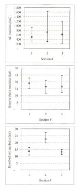
Figure C-19 Variability of the Backcalculated Moduli for Site #8
