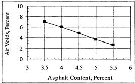
Figure 2.17 Example of test property curves for hot-mix design data for Marshall method
