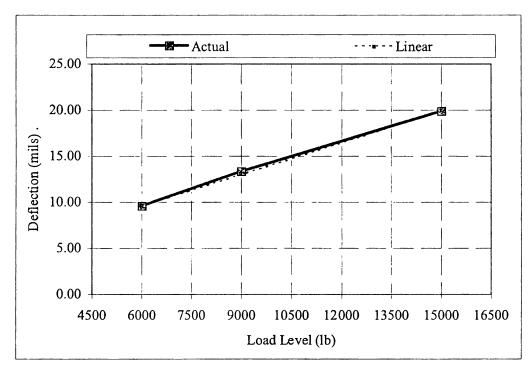
Figure 4.4 Deflection data vs. load level linearity plot for test site 1
