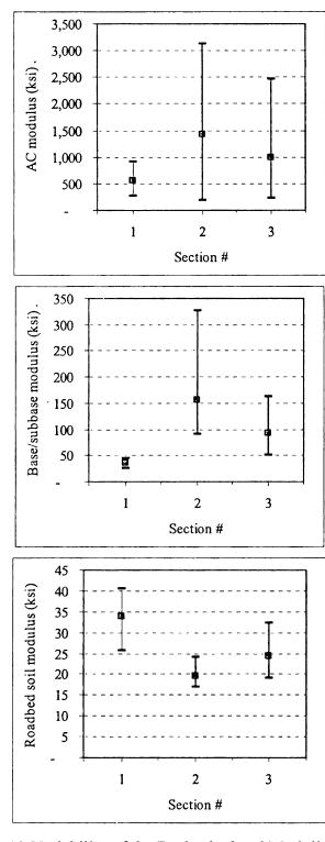
Figure C-12 Variability of the Backcalculated Moduli for Site #1
