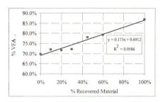
Figure E-15 VFA versus percent recovered material for DW-M (Superpave Mixture)
