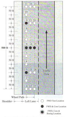
Figure 3.4 FWD test, coring and boring locations for an AC section
