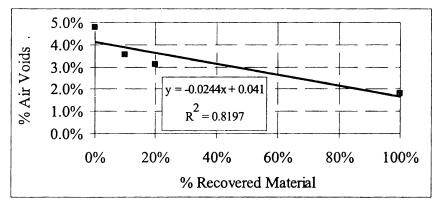
Figure E-12 Air voids versus percent recovered material for DB-N (Superpave Mixture)
