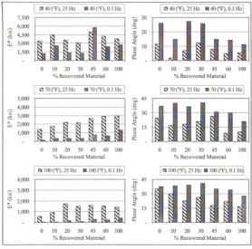
Figure E-24 Variability of E\* and  $\delta$  for the same temperature and frequency for wearing course Deena + Mandra blends
