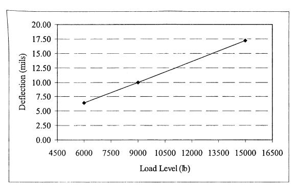
Figure C-3 Deflection Data vs. Load Level Linearity Plot for Site #4
