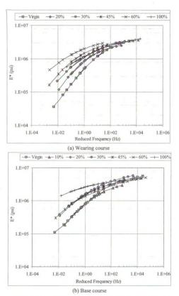
Figure 4.25 Master curve for the Deena + Nowshera recycled mixtures
