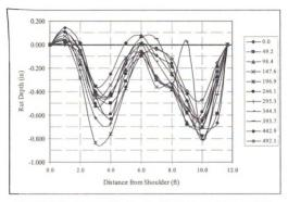
Figure B-17 Horizontal profiles from 0 - 492.1 ft along test site 7, section 1
