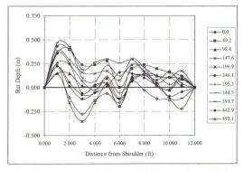
Figure B-22 Horizontal profiles from 0 - 492.1 ft along test site 8, section 3
