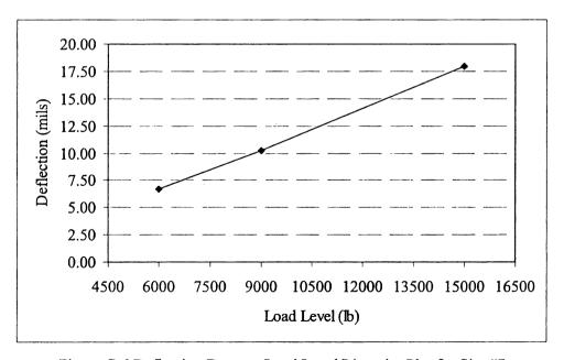
Figure C-6 Deflection Data vs. Load Level Linearity Plot for Site #7
