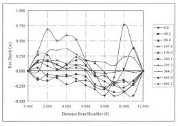
Figure B-6 Horizontal profiles from 0 - 492.1 ft along test site 2, section 3
