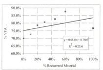
Figure E-16 VFA versus percent recovered material for DW-N (Superpave Mixture)
