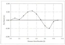
Figure B-26 Average profile of test site 1
