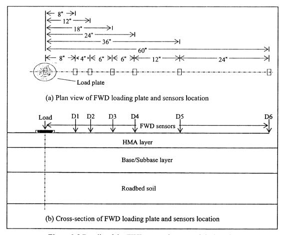
Figure 3.8 Details of the FWD sensor layout and designation
