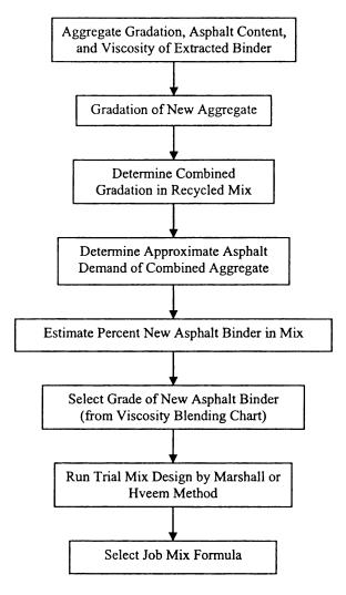
Figure 2.19 Flow chart for mix design procedure
