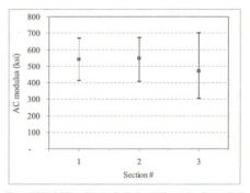
Figure 4.8 Variability of the backcalculated AC modulus for test site 3
