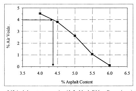
Figure 3.13 Asphalt content versus air voids for Marshall Margalla wearing mixtures
