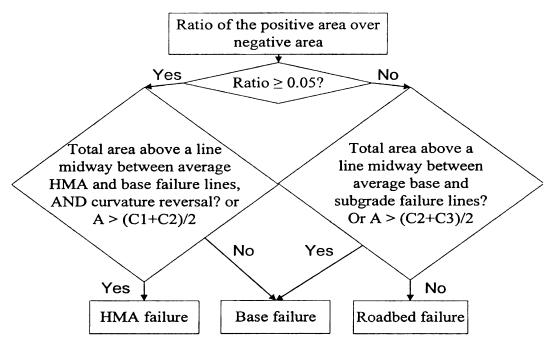
Figure 2.14 Conditions for determining the rutting seat (NCHRP 2002)
