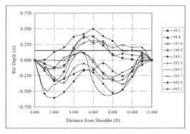
Figure B-12 Horizontal profiles from 0 - 492.1 ft along test site 5, section 2
