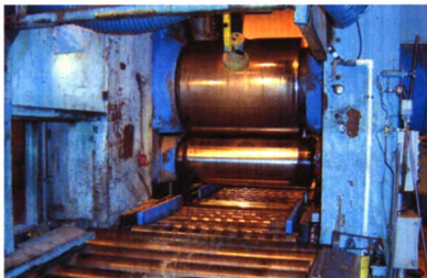
Figure 3.6. Rolling mill at Manufacturing Sciences Corporation (Oak Ridge, TN) facility. (Courtesy of Dr. Tamirisakandala)
