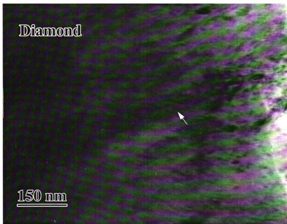
FIGURE 5.31 : DARK FIELD TEM IMAGE Sample: Deposition pressure=120 Torr, Ar/H 2 /CH 4 =100/4/1 sccm and deposition time=8 hours by system II
