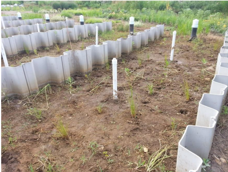
Figure 67. Bioretention Bays with white PVC water content monitoring ports installed
