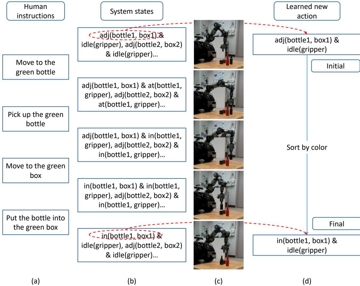
Figure 3.5: Programming the skill of "Sorting by color" with step by step instructions. (a) Natural language commands given by the instructor. (b) Initial system state and temporal states after each implementation. (c) Snapshots of robot execution corresponding to system state in column (b). (d) The representation of learned new behavior.
