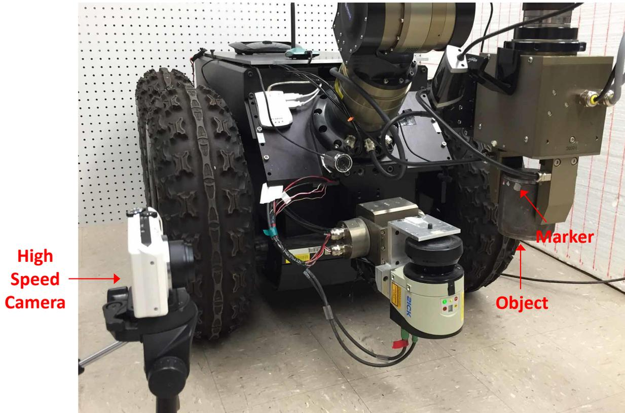
Figure 5.5: This system is used to evaluate the performance of the second approach. White markers are stuck to the cylinder's surface and facing the camera lens.
