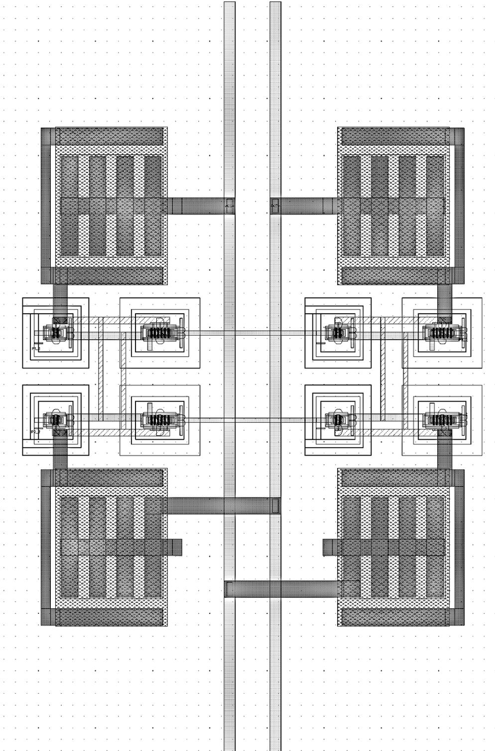
Figure A-10. Layout of a Two-Stage Rectifier
