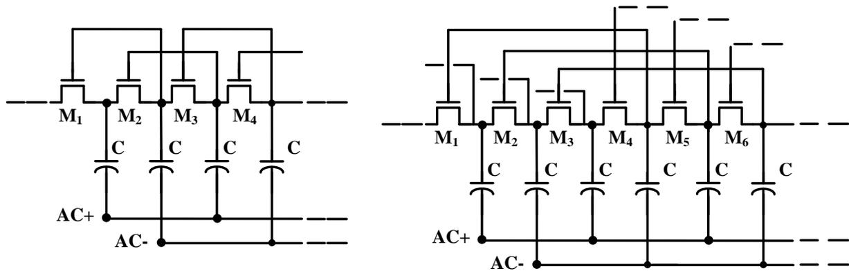
**Figure 2-5. Single Order Self Compensation Method (left) and Higher Order Self Compensation Method (right)**
