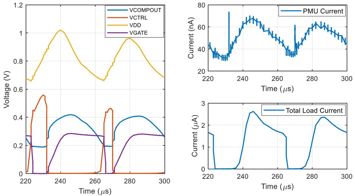
**Figure 3-10. Respective Voltage and Current Levels in Power Management Unit and Load**
