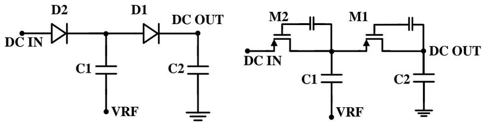
Figure 2-3. A Conventional Voltage Doubler Rectifier (left) and a PMOS Floating-Gate Rectifier (right)
