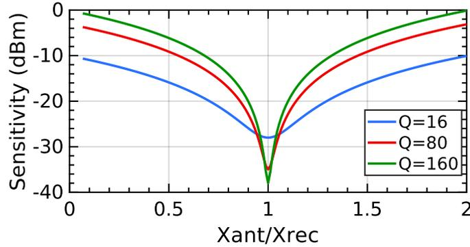
**Figure 3-2. Mismatch in Imaginary Impedances vs. Sensitivity for Different Q-factor Values**
