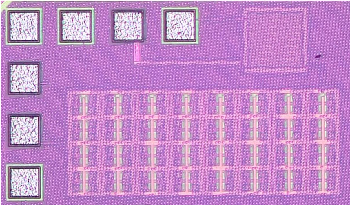
Figure 4-23. Design 8 Micrograph
