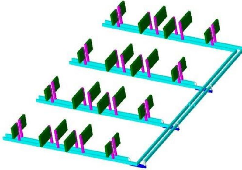
Figure 4-1. Electromagnetic Simulation Layout of the Input Lines
