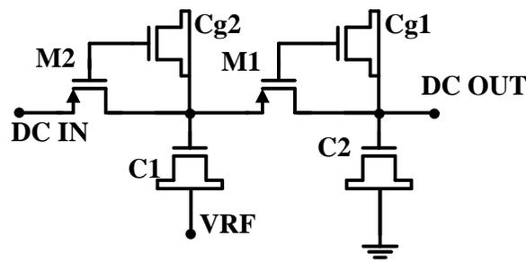
Figure 2-4. Transistor Level Schematic of PMOS Floating-Gate Rectifier
