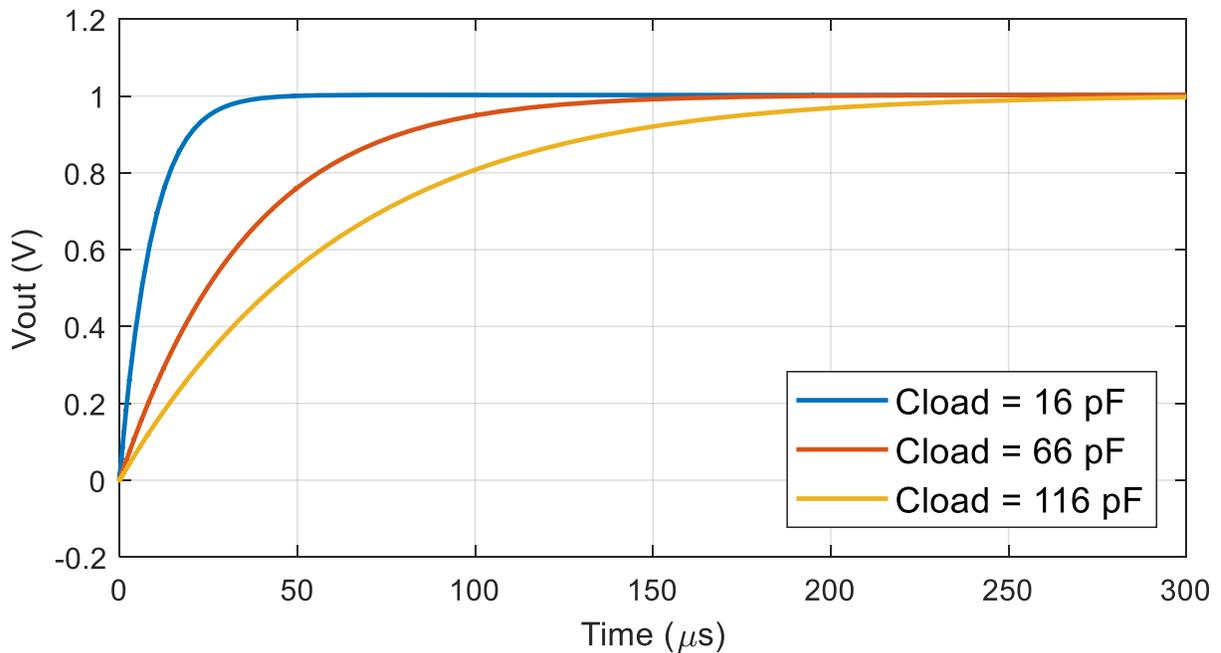
**Figure 3-8. Output Voltage Transient Waveform for Different Load Capacitances**
