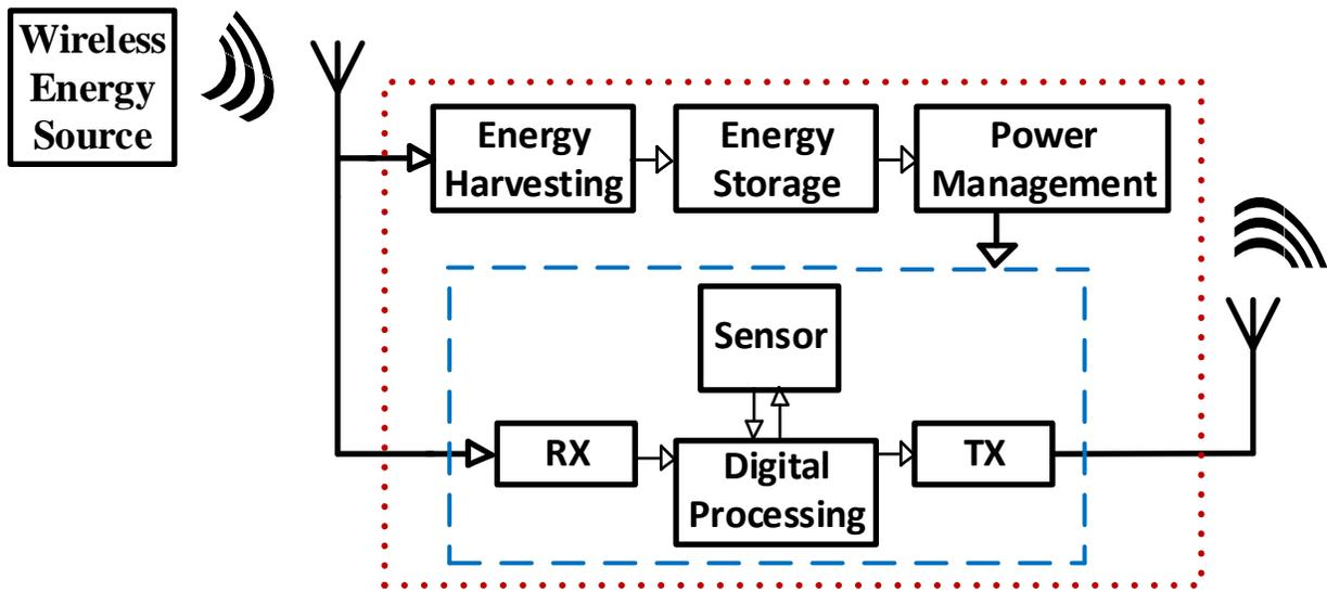
Figure 2-1. Energy Harvester with Sensor Nodes
