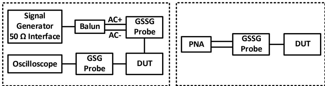
**Figure 4-2. Measurement Setups for Output Voltage Waveform (left), and Input Impedance (right)**
