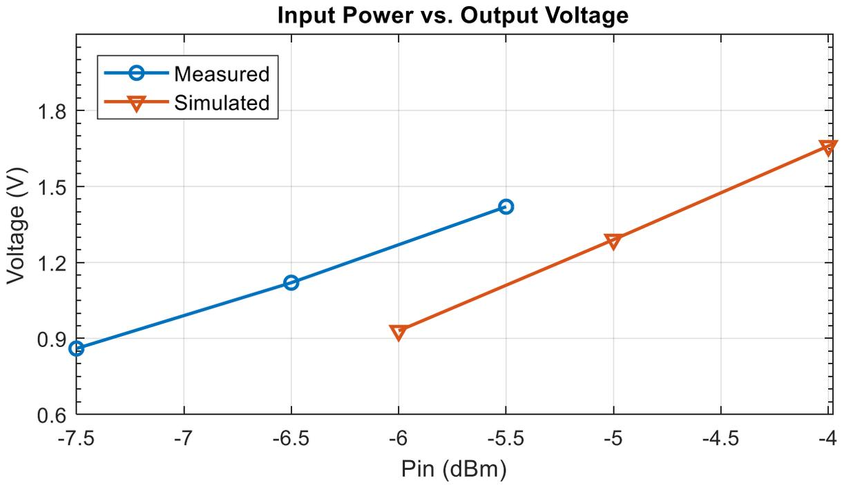
**Figure 4-9. Measurement and Simulation Input Power vs. Voltage Levels of Design 3**
