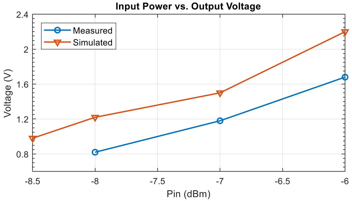
Figure 4-19. Measurement and Simulation Input Power vs. Voltage Levels of Design 7
