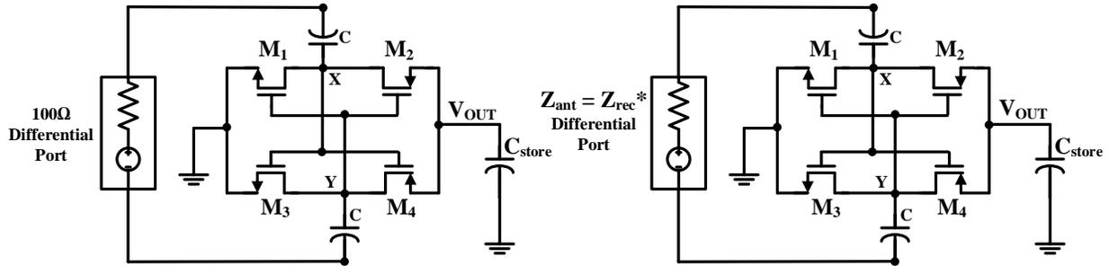
**Figure 3-5. Impedance Analysis Setups for Single Stage Topology**
