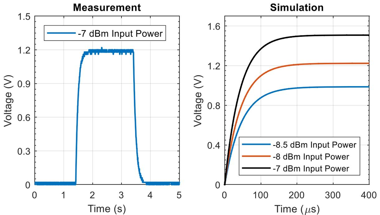
Figure 4-18. Measurement and Simulation Output Transient Voltage Waveforms of Design 7
