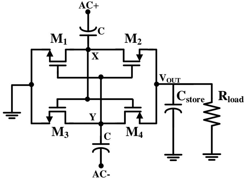
Figure 2-6. A Differential Drive Rectifier Circuit
