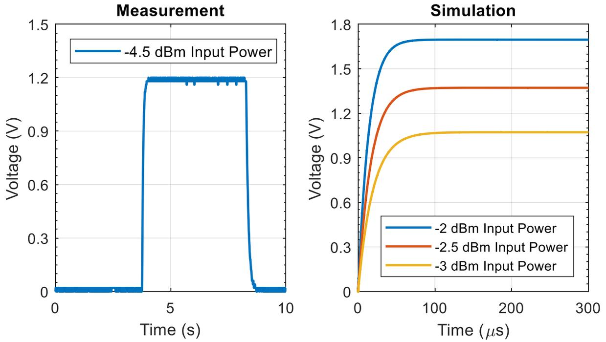
Figure 4-5. Measurement and Simulation Output Transient Voltage Waveforms of Design 2
