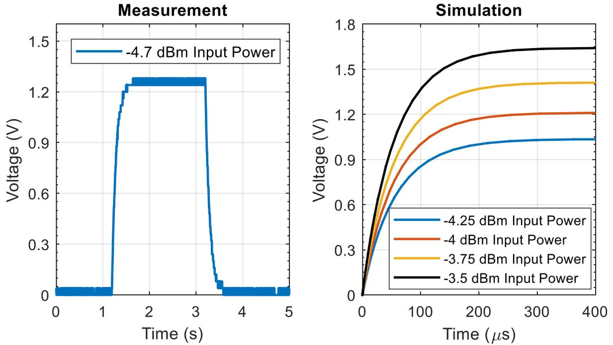
Figure 4-21. Measurement and Simulation Output Transient Voltage Waveforms of Design 8
