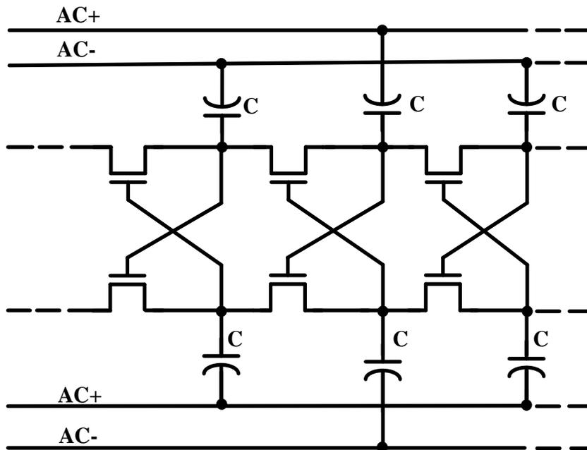
Figure 2-7. Threshold Self Compensation in Differential Drive Topologies
