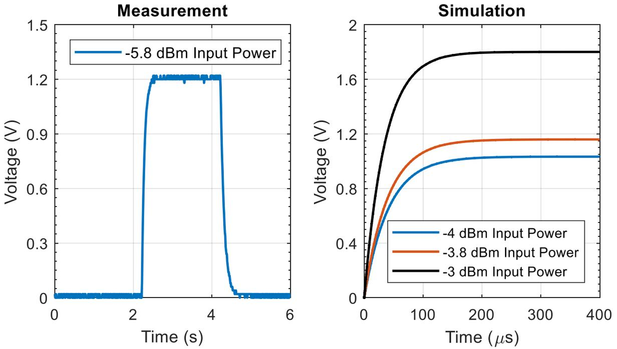
Figure 4-13. Measurement and Simulation Output Transient Voltage Waveforms of Design 5
