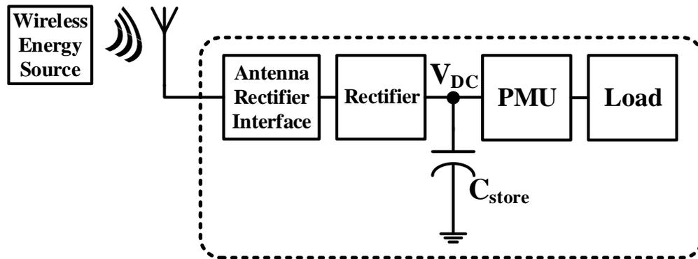
Figure 1-1. Energy Harvester Building Blocks
