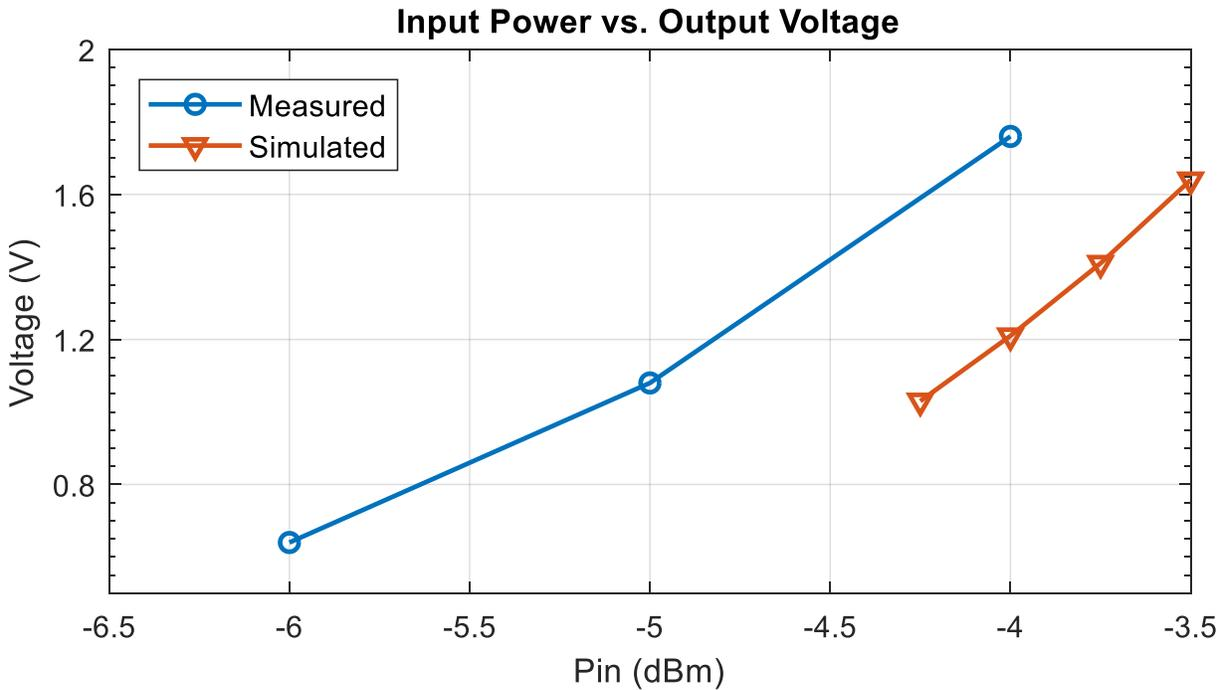
Figure 4-22. Measurement and Simulation Input Power vs. Voltage Levels of Design 8
