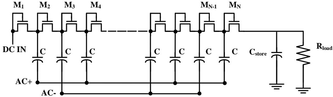
**Figure 2-2. Conventional Multi-Stage Dickson Rectifier**
