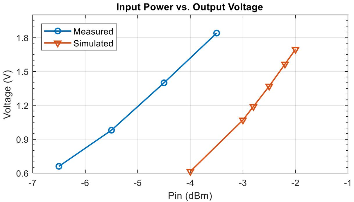
Figure 4-6. Measurement and Simulation Input power vs. Voltage Levels of Design 2
