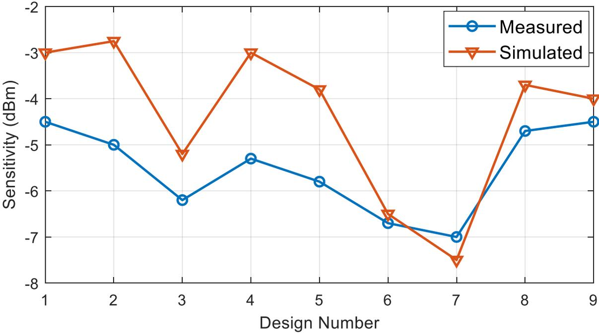
**Figure 4-26. Measured and Simulated Sensitivity Values for 1.2 V Output Voltage After Loss Calibration based on 50 Ω Single Ended Input Source and Balun Setup**
