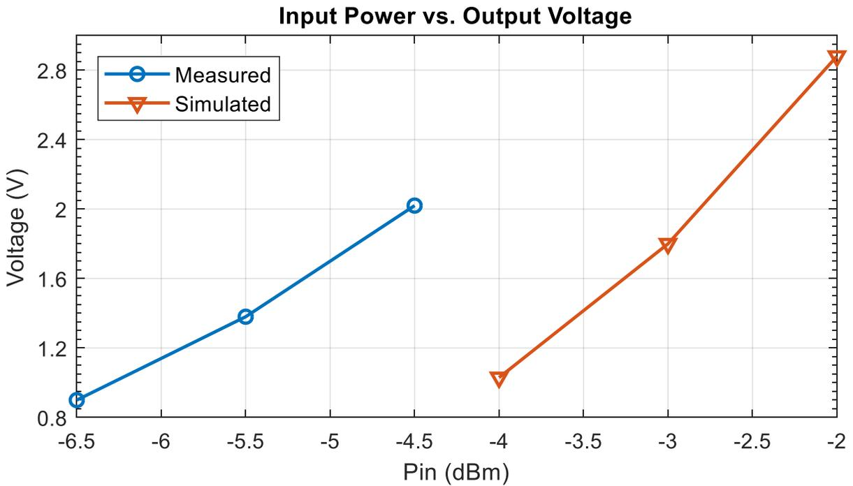
Figure 4-14. Measurement and Simulation Input Power vs. Voltage Levels of Design 5
