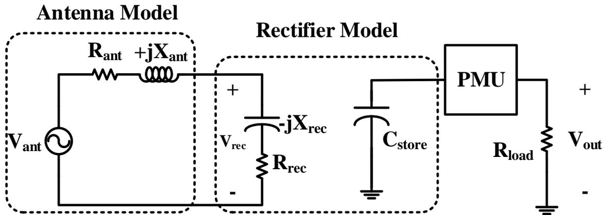
Figure 3-1. Antenna–Rectifier Interface
