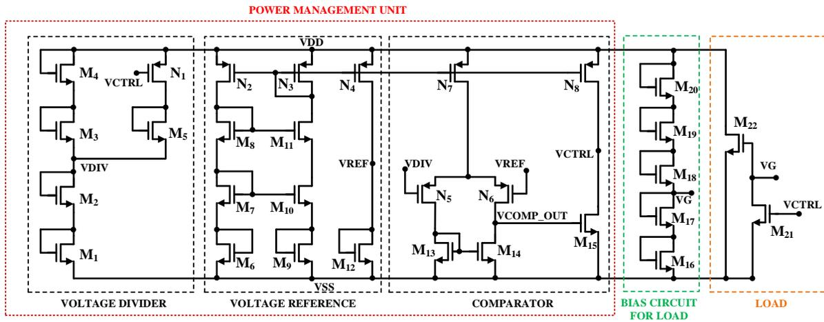
**Figure 3-9. Power Management Unit with Load**
