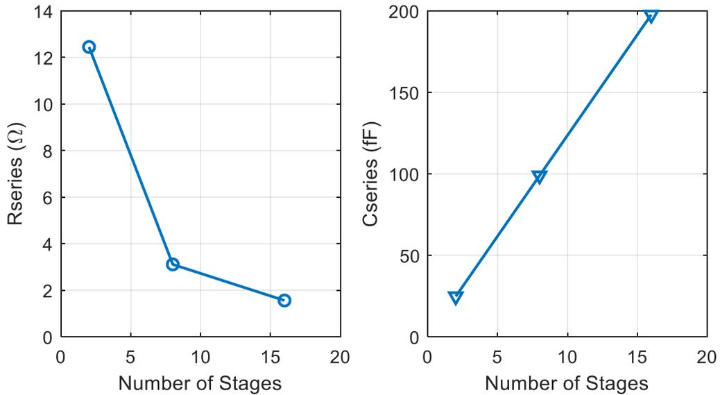
Figure 3-7. Rectifier Input Impedance for Different Number of Stages
