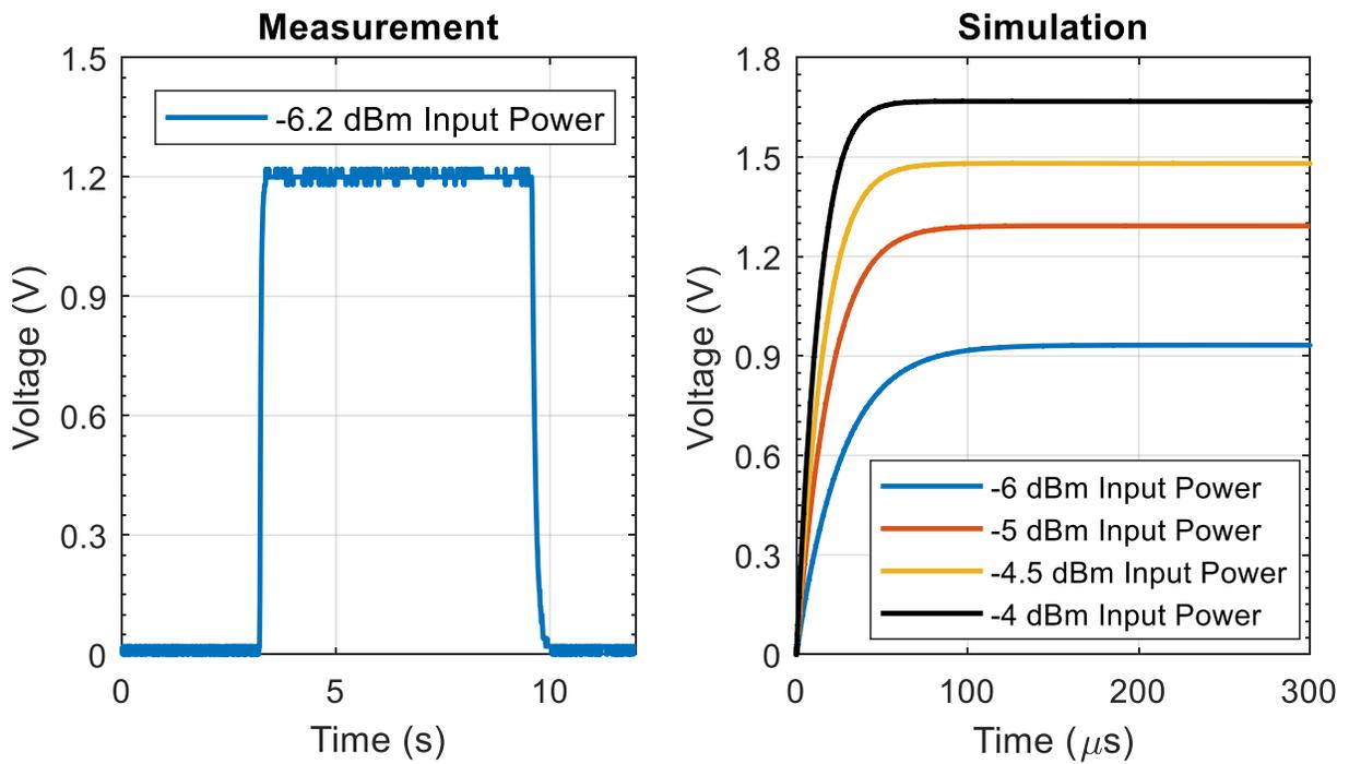
Figure 4-8. Measurement and Simulation Output Transient Voltage Waveforms of Design 3
