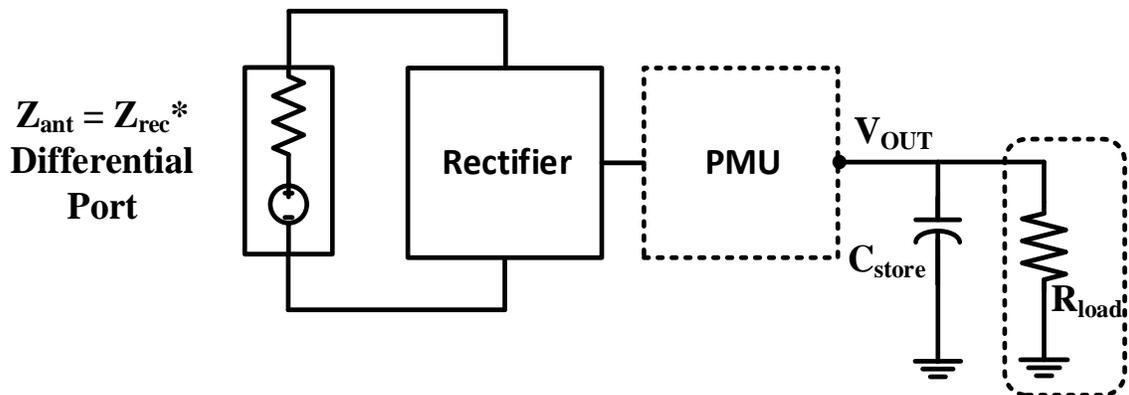
**Figure 4-27. Simulation Setup for Rectifier and Antenna Conjugately Matched Energy Harvesters**
