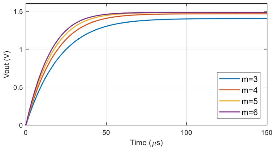
**Figure 3-4. Output Voltage Transient Waveform for Different Device Sizes**
