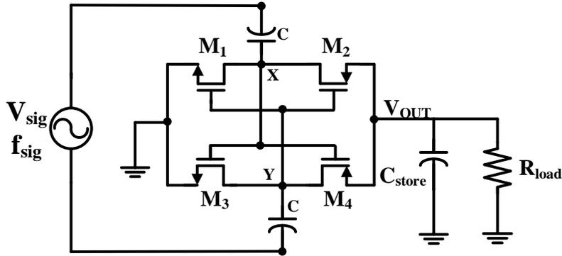
**Figure 3-3. Analysis Setup for a Single Stage Topology**
