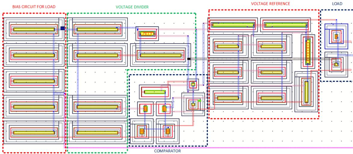
Figure 3-12. Layout of Power Management Unit with Load
