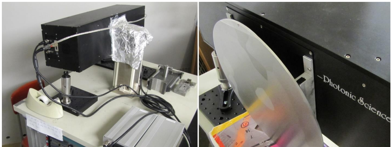
Figure 22: Laue camera equipped with area detector, showing how an ingot slice was mounted to determine crystal orientations [Figure 3 in reference [122]].
