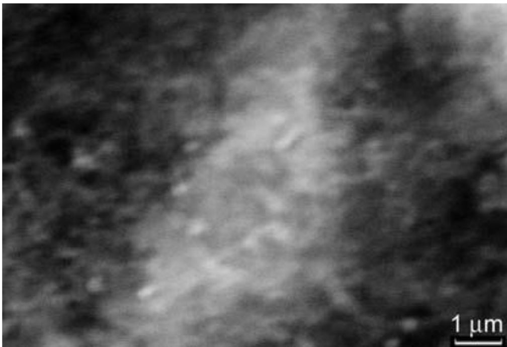
Figure 9: Electron channeling contrast image of a sample from an as-received Nb ingot showing contrast arising from dislocations [Figure 8 in reference [24]].
