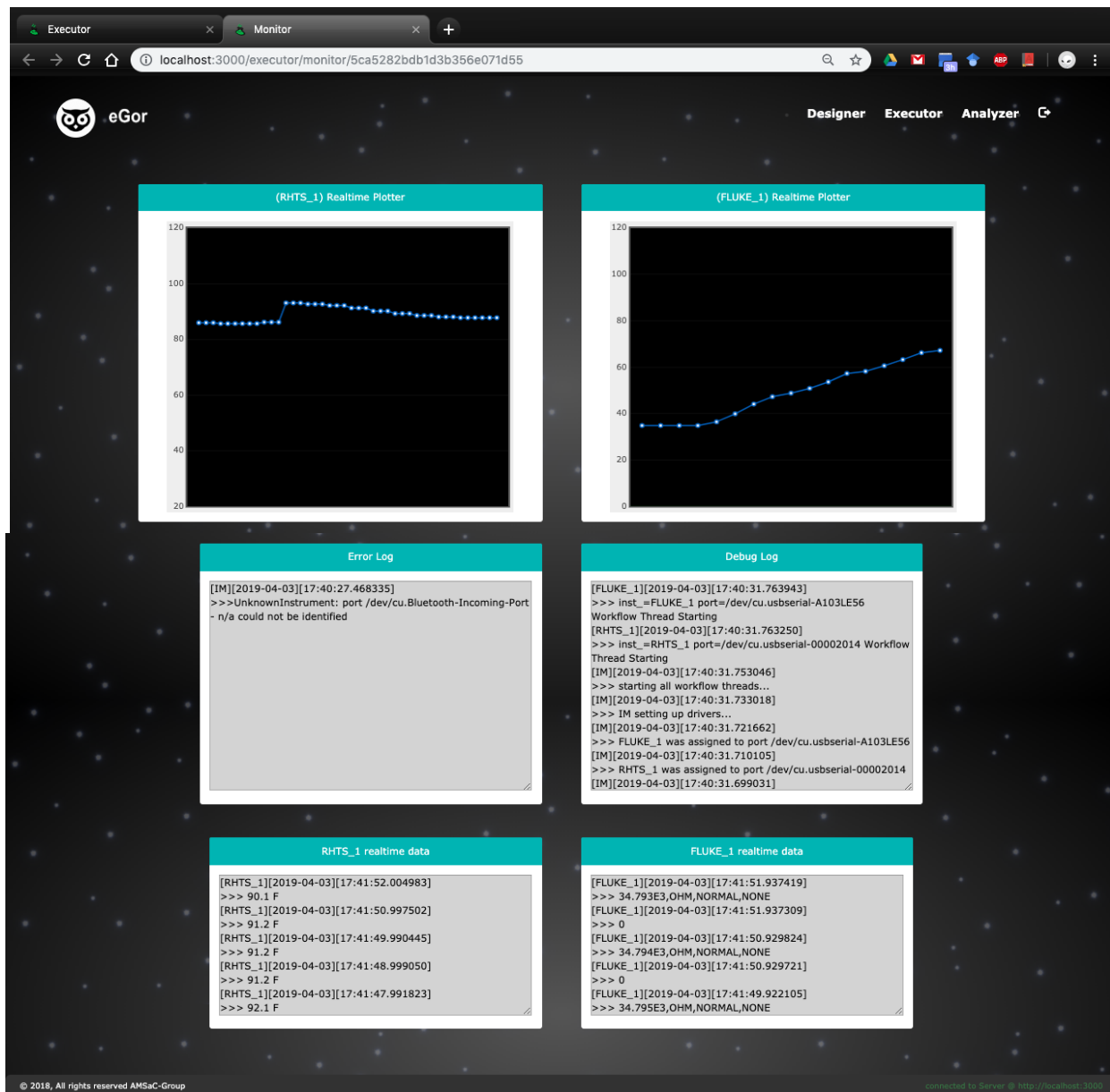
Fig. 4. 21 Snapshot of the Analyzer browser tool displaying run time error and debug logs, timestamped raw data logs, and plots of temperature, humidity, and digital multimeter measurement data.
