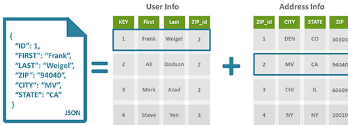
Fig. 2. 4 Document based non-relational database model (left) vs. table based relational database model (right)
