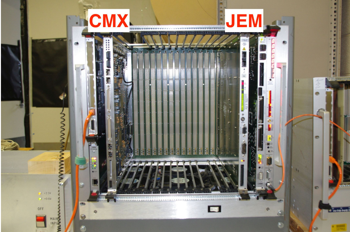
Figure J.4: One of the production CMX boards and a JEM in the test crate located in the HEP lab on the Michigan State University campus. The JEM was used to test the functionality of the backplane. As only one JEM was available during testing, after each test it was shifted to another slot in order to test all 400 pins in the backplane.
