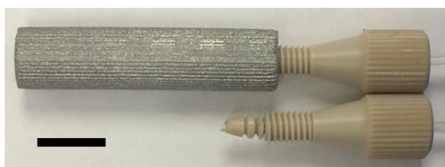
Figure 2.6 A photograph of the SS PC (with BN) connected with the commercially available PEEK fitting (for 1/16" tubing, IDEX Health & Science). Scale bar = 1 cm.
