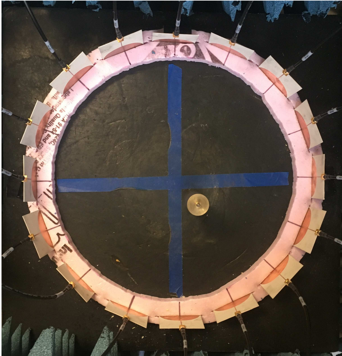
Figure 3.1 Test setup of a brass cylinder being imaged by the microwave tomography system.
