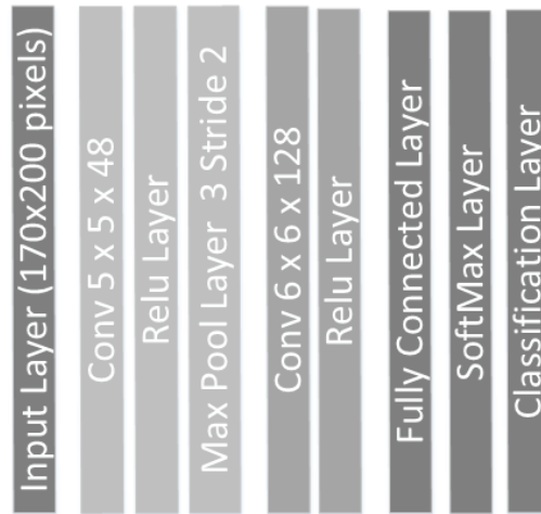
Figure 2.15: CNN architecture for gender and race prediction from a NIR ocular image.
