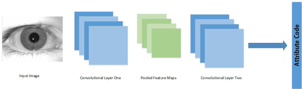
Figure 5.2: Attribute code generation. An NIR ocular image is applied to the input of a Convolutional Neural Network trained to predict that attribute, the activation from the second convolutional layer is reshaped into a single one dimensional feature vector.
