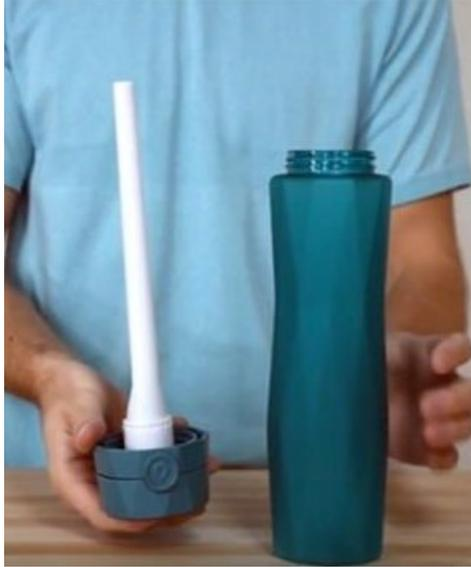
Figure 2-1: Image of an Augmented Container Using an Insertable Capacitive Sensor [23]
