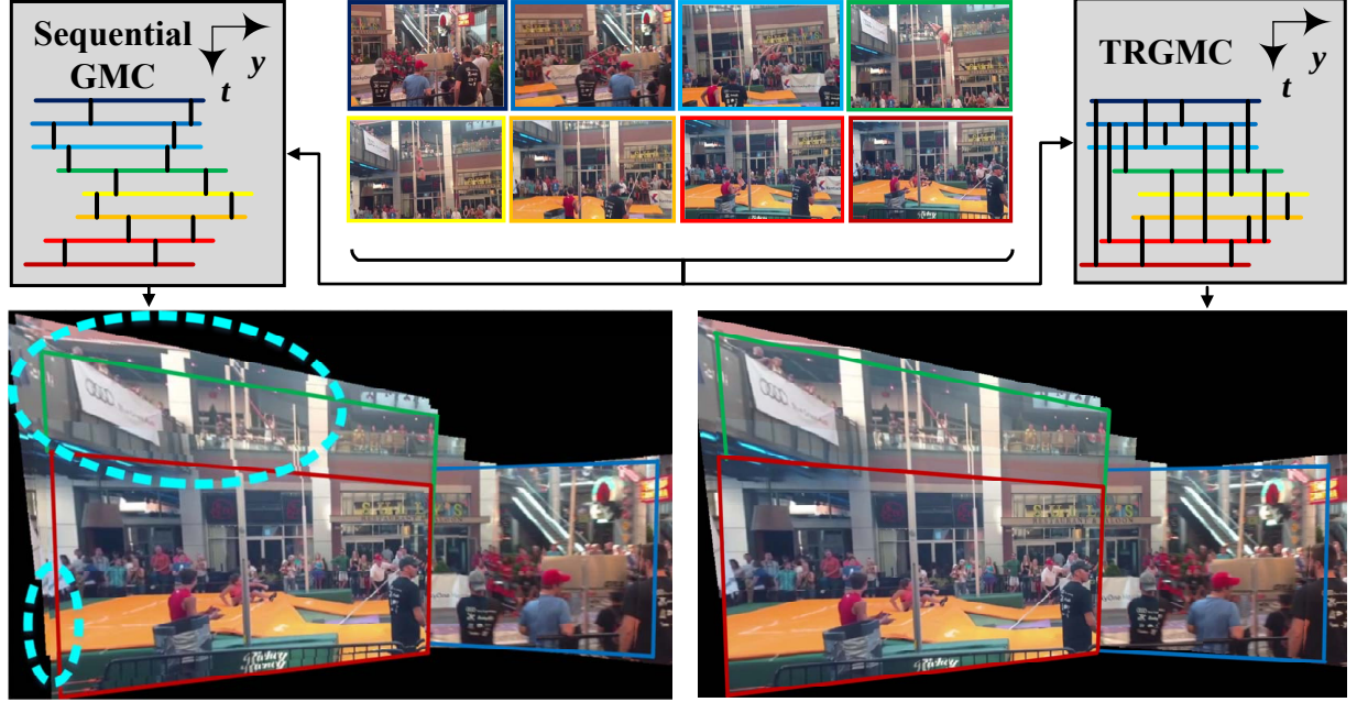
Figure 4.1: Schematic diagrams of proposed TRGMC and existing sequential GMC algorithms, and resultant motion panorama for a video shot by panning the camera up and down. Background continuity breaks easily in the case of the sequential GMC [88].
