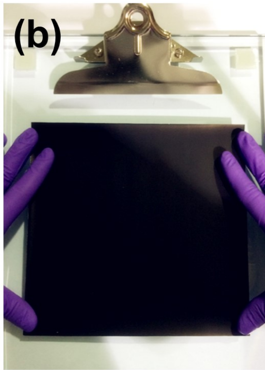
Figure 4.12 (a) Convenient bar-coating process for fabricating electrodes over large-area PPFES. (b) Large-area FENG fabricated with simple bar-coating technique.
