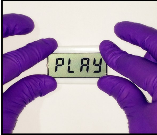
Figure 4.18 A self-powered LCD touch screen which is able to scavenge energy from finger touch. Word "PLAY" is displayed on the screen by touching a small area of the corners by the user.
