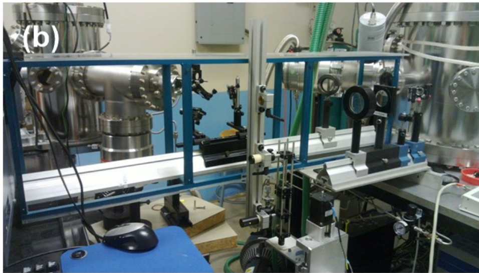
Figure 3.3 Photograph of PLD system for piezoelectric AlN thin film growth. (a) Ultra-high vacuum chamber. (b) Optical components.
