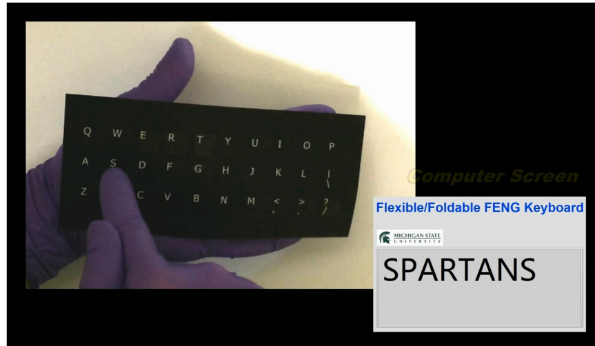
Figure 4.20 Real-time keystroke tracing and recording. As the user types the word “SPARTANS”, the output is displayed on a computer monitor.
