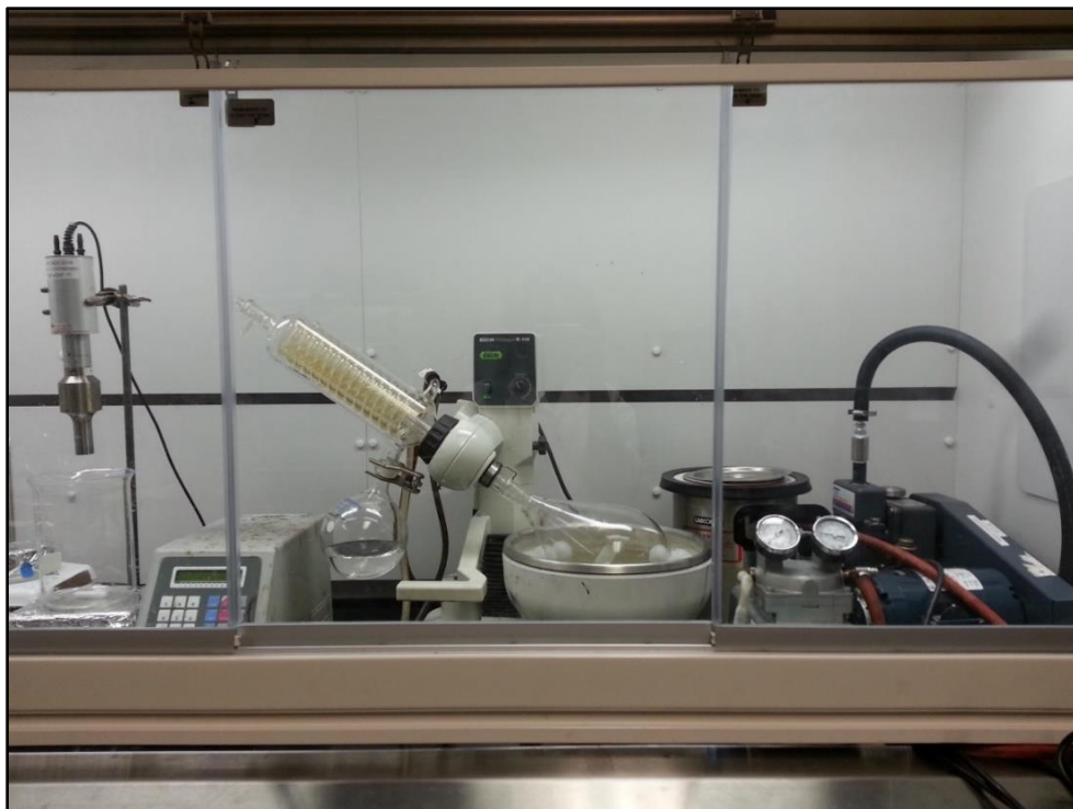
Figure 2.1: Solvent exchange process using a rotary evaporator.
