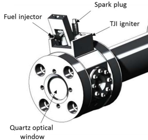
Figure 2-4 Enlarged view of RCM head fitted with optical window and TJI igniter.
