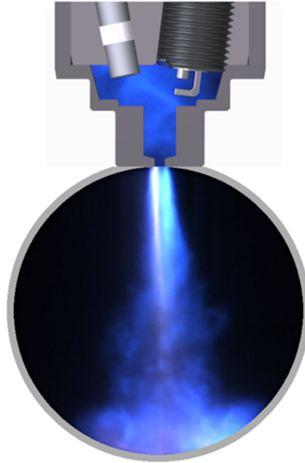
Figure 1-1 Illustration of TJI with a single orifice nozzle as visualized from a RCM experiment [36].
