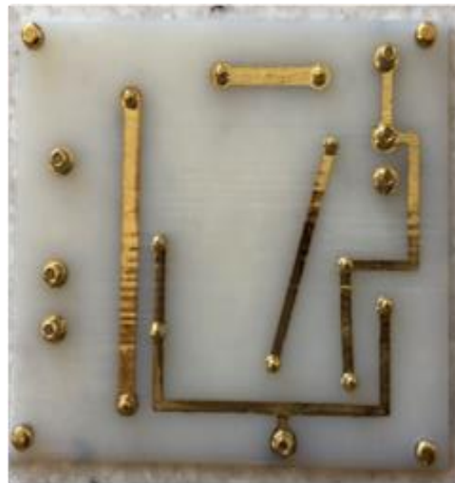
Figure 4. 6: a) Concept diagram of using PVD (e-beam evaporation) on 3D-printed microsystem, and b) real image of the deposited Ti/Au on two layers microsystem.
