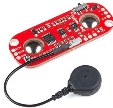
Figure 3. 2: off-the-shelf biomedical signal acquisition devices: A) MG-300, B) Mindwave mobile from NeuroSky, and C) MyoWare sensor from Advancer Technologies.
