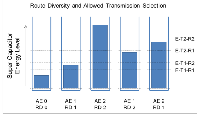
Figure 5.2. Routing Decision based on Energy Levels
