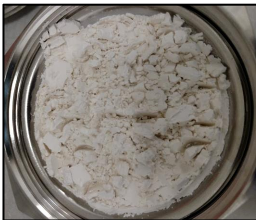
Figure 12. Typical appearance of fine soy protein powder accumulated in the secondary collector after spray drying.
