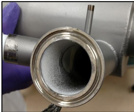
Figure 15. Nozzle shield with deposited soy protein powder after spray drying.
