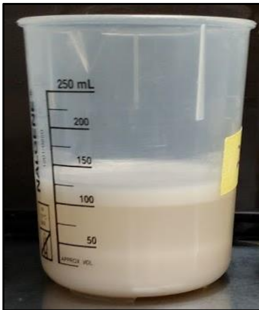
Figure 3. Separation of a 10% w/w soy protein isolate (SPI) solution into watery and paste-like phases after blending.
