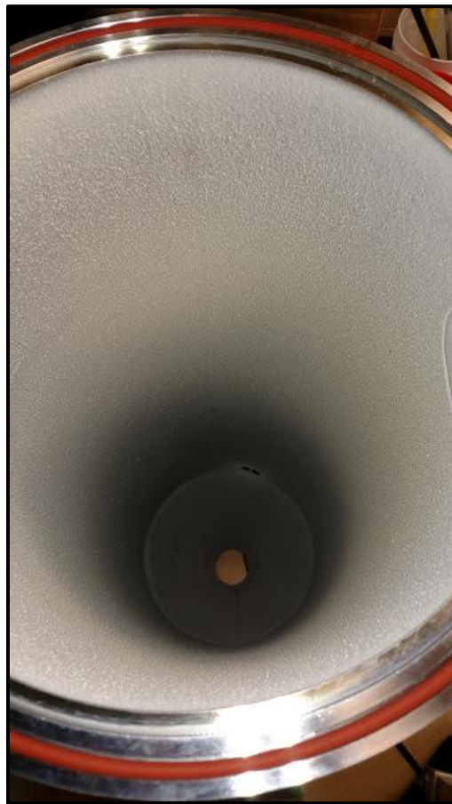
Figure 14. Top-down view of the spray drying chamber with deposited soy protein powder after spray drying.
