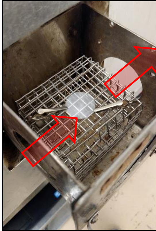
Figure 5. Nylon mesh attached to wire rack placed inside a convection oven sampling port. Arrows indicate the direction of heated airflow.
