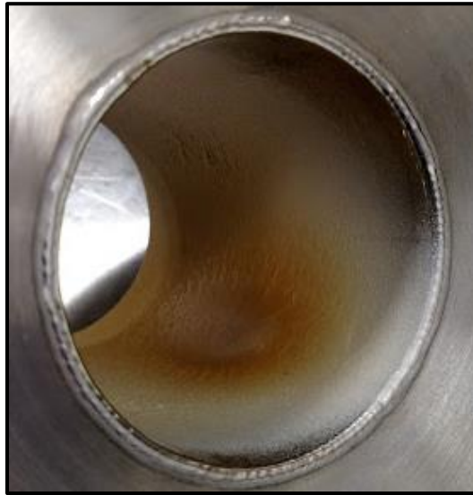
Figure 15. Nozzle shield with deposited soy protein powder after spray drying.
