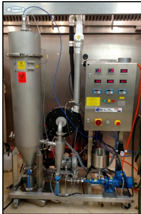
Figure 2. FT80 Tall-form Spray Drier housed in the Biosafety Level 2 pilot plant facility at Michigan State University.
