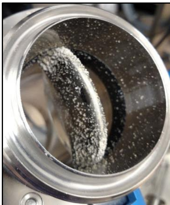
Figure 13. Typical appearance of accumulated coarse soy protein powder in the primary collector after spray drying.
