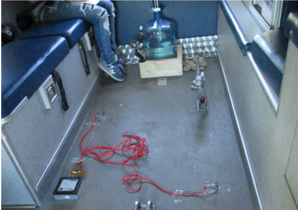
Figure 50. Location of tri-axial accelerometers and Saver on the floor of an ambulance.
