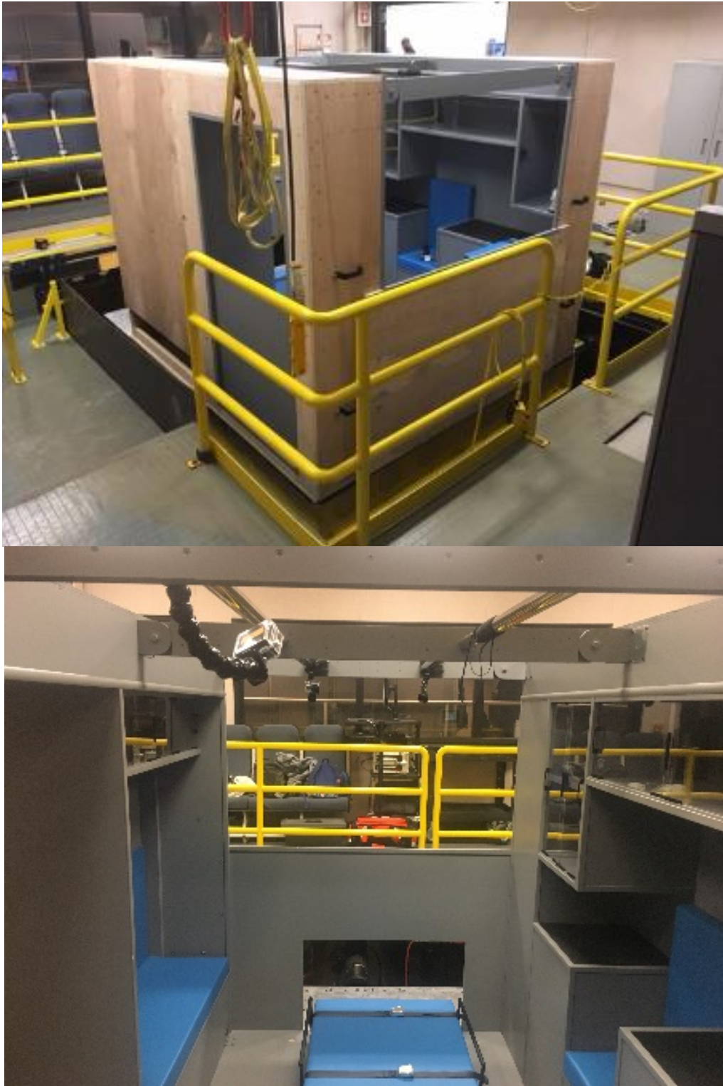
Figure 57. The ambulance simulator mounted on the vibration table at Adient
