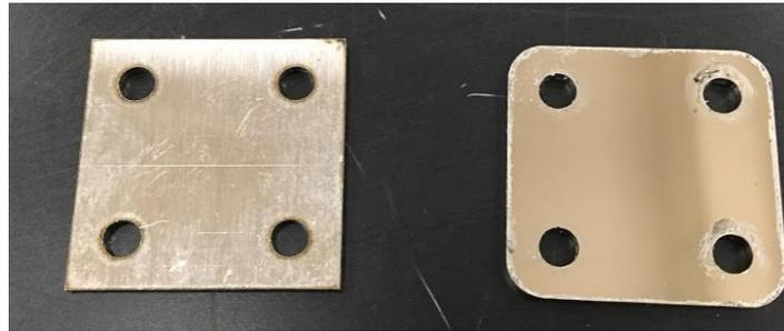
Figure 9 Stainless steel 304 #4 brushed (left) #8 mirror finish (right) coupons used in the centrifuge experiment for measuring critical attachment force of *Salmonella* Enteritidis PT30 in a low-moisture environment.
