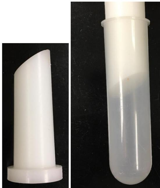
Figure 10 Centrifuge sample holder (left) inserted in centrifuge tube (right) used for a centrifuge block (SS-34). Fabricated in the Department of Biosystems and Agricultural Engineering Shop, Michigan State University (East Lansing, MI).
