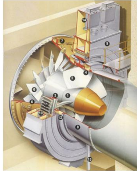
Figure 1.8. An example layout of the Straflo turbine for low head application [34]
