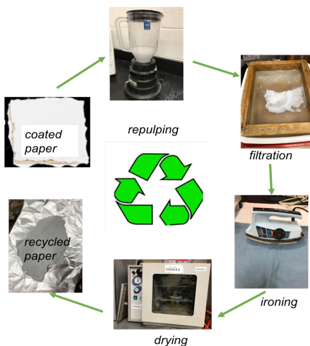
Scheme 5. 2 Illustration of the pulp recycling process for the coated paper.
