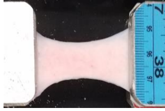
Figure 14. A UB sample mounted on the uniaxial machine, submerged in Krebs solution.
