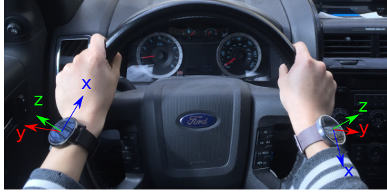
Figure 3.6: The 3-axis coordinate system for the accelerometers and gyroscopes on the smartwatches
