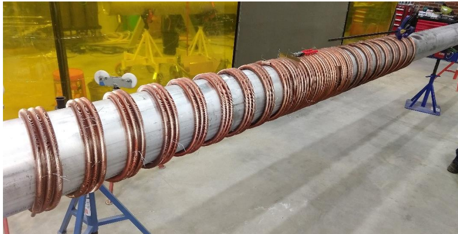
Figure 4.3: Coiled tubes carefully spaced out on the mandrel
