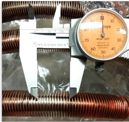
Figure 3.3: Finned tubes being measured on reception
