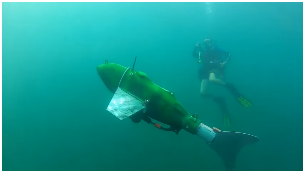
Figure 3.3: A gliding robotic fish prototype during field experiments in Higgins Lake.
