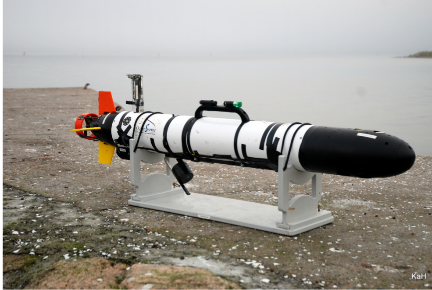
Figure 1.2: Example of OceanServer Iver2 propelled AUV used in acoustic telemetry [18].
