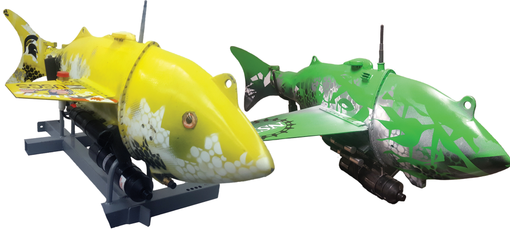
Figure 2.4: Second-generation (Grace 2) prototypes of gliding robotic fish.
