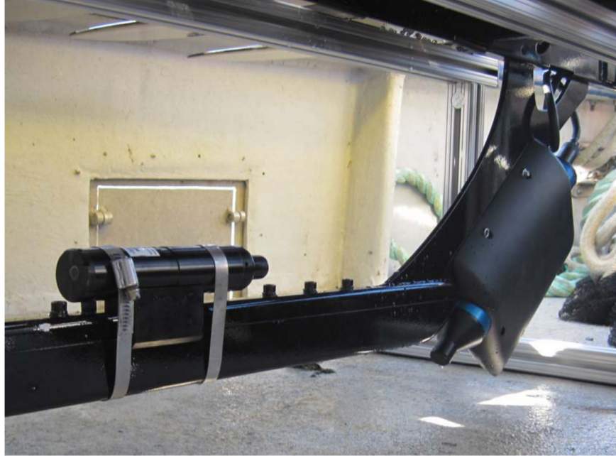
Figure 1.3: Exampe of a Liquid Robotics wave glider AUV used in acoustic telemetry [17].
