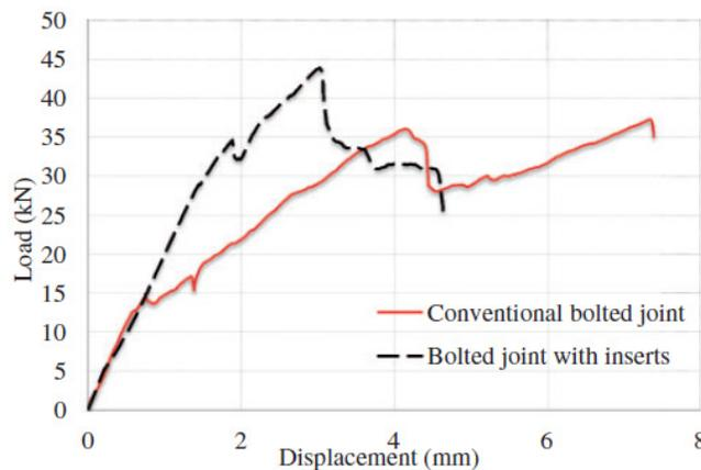
Figure 1-11: Load–displacement curves for a conventional bolted joint and a joint with inserts [17].
