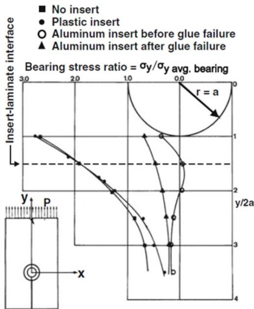
Figure 1-1: Bearing stresses with inserts[6][19].
