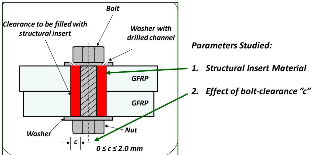
Figure 1-3: Schematic of parameters studied in this work.
