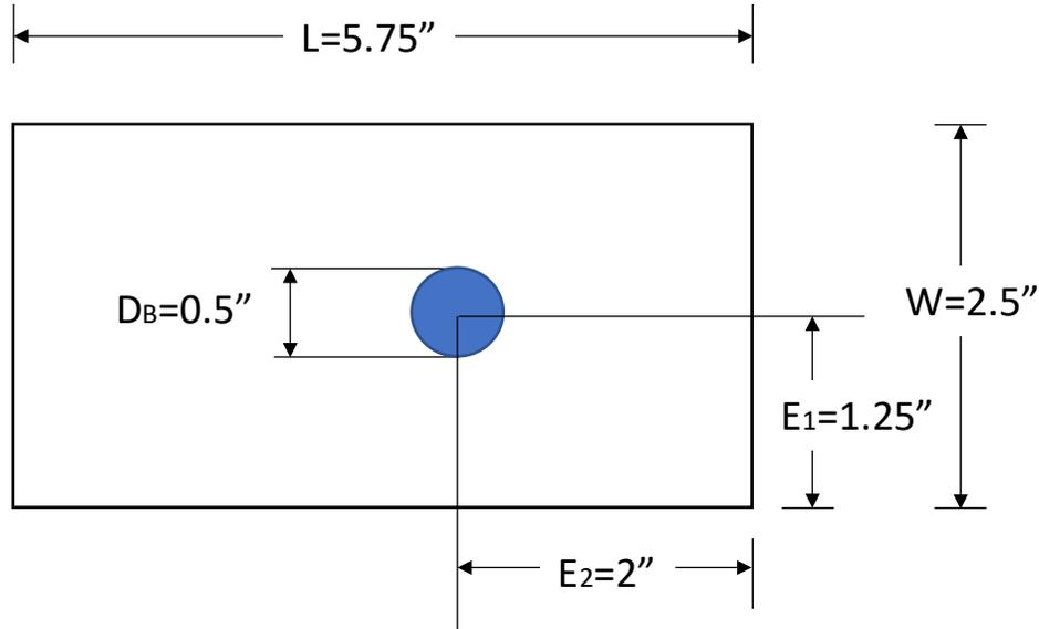
Figure 2-3: Dimension of GFRP specimen.
