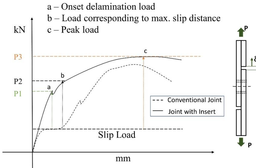
Figure 3-3: Schematic of lap-shear behavior of conventional and hybrid joints.
