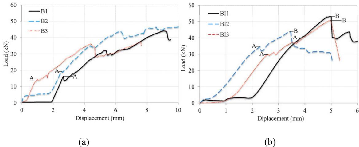
Figure 1-10: Load–displacement curves for; (a) conventional bolted joints (B1-B3), (b) bolted joints with inserts (BI1-BI3) [17].
