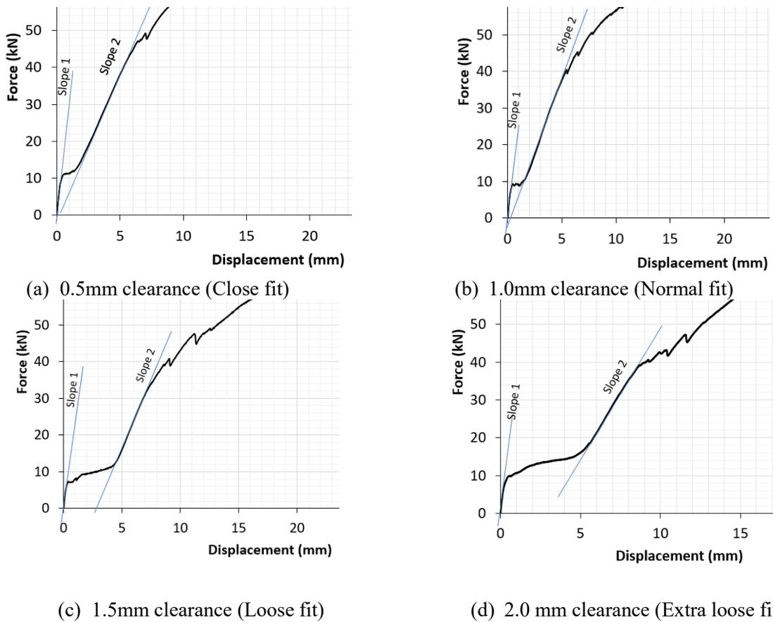
Figure 5-4: Stiffness changes pre- and post-slip in conventional bolted joints with varying bolt-hole clearances.
