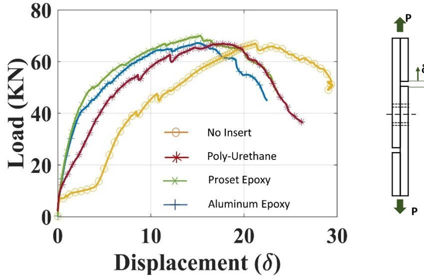
Figure 4-4: Load-displacement response for hybrid fastening system with various structural inserts (bolt-clearance = 1.5 mm.)
