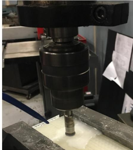
*Figure 2-9: Drilling process using 1/2" diamond core drill.*
