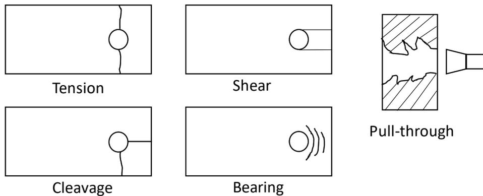
Figure 1-4: Failure modes in composite bolted joints.
