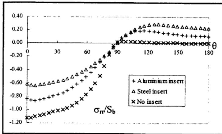
Figure 1-9: Normalized radial stress distribution for CFRP laminates bolted joint [24].
