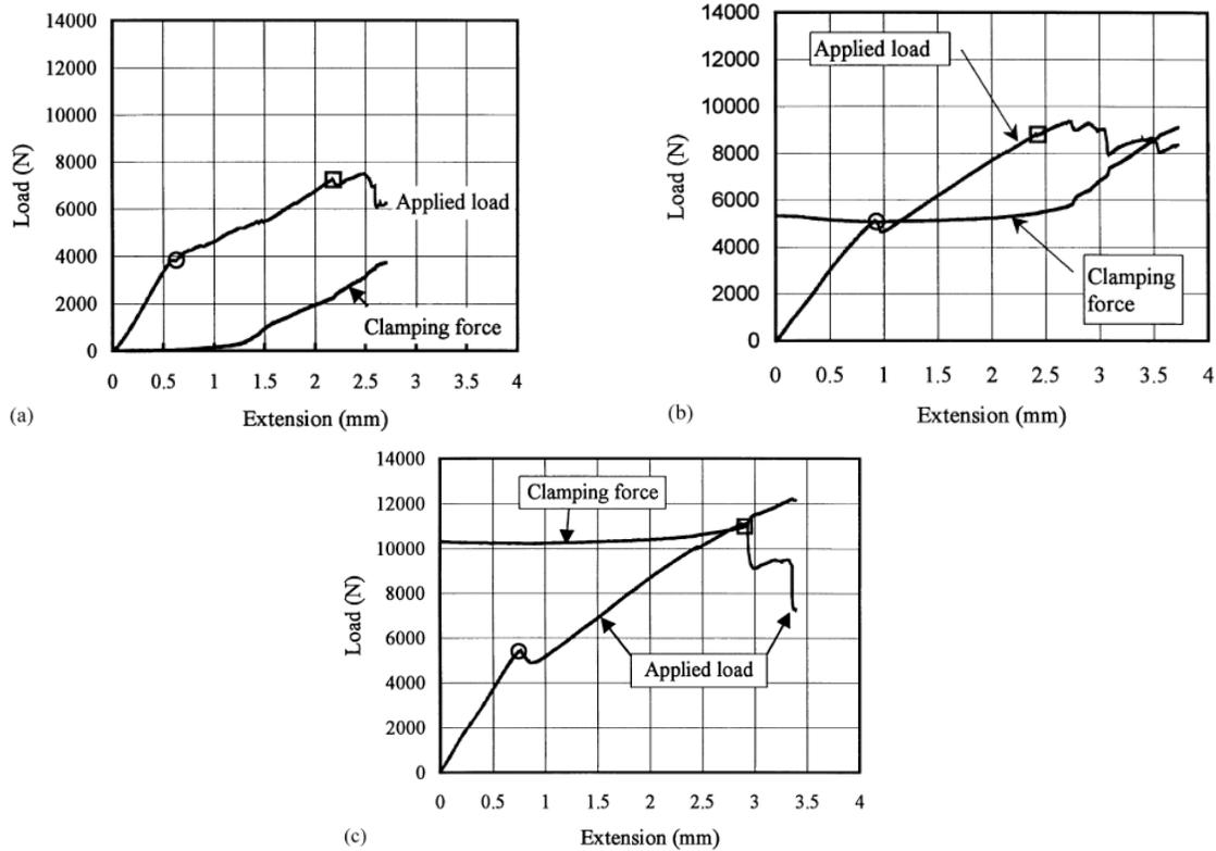
Figure 1-19: Applied load and clamping force versus the axial extension for case (a): specimen 3 with an applied torque of 0 N m (finger tight) (a); specimen 4 with an applied torque of 6.4 N m (b); specimen 8 with an applied torque of 12.88 N m (c).[29].
