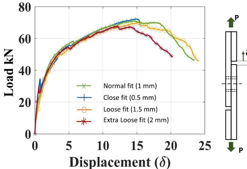
Figure 5-9: Load-displacement response of hybrid joints with Proset epoxy insert and varying bolt-hole clearances.
