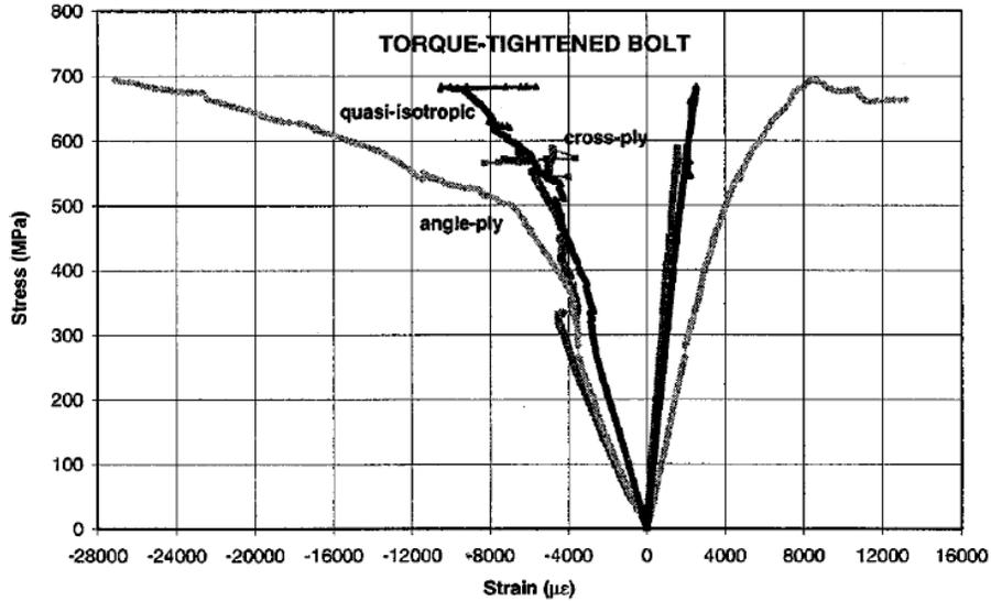
Figure 1-16: Stress vs local strain curves for 20Nm torque tightened bolt [13][14].
