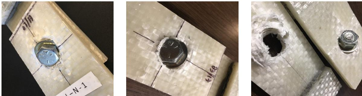
Figure 4-3: Post failure images of conventional bolted joints.
