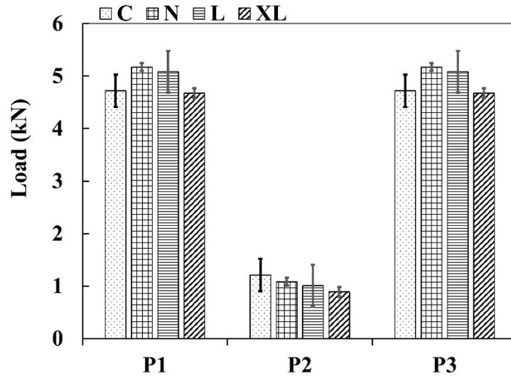
Figure 5-14: Effect of clearance on hybrid joints with poly-urethane epoxy inserts.
