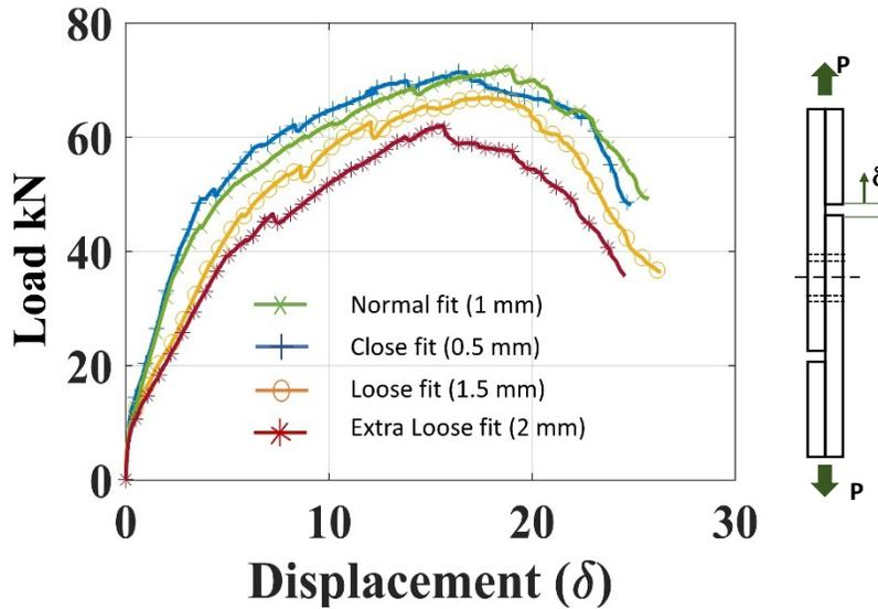
Figure 5-13: Load-displacement response of hybrid joints with polyurethane epoxy insert and varying bolt-hole clearances.
