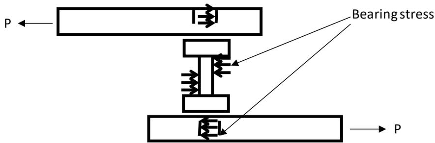
Figure 1-6: Bearing stress in bolted joint.
