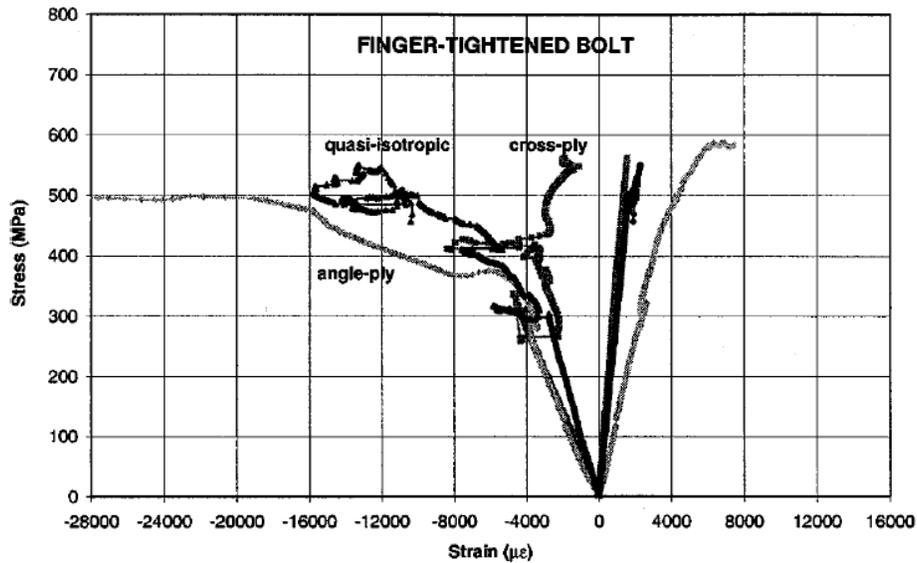
Figure 1-15: Stress vs local strain curves for finger tightened bolt [13][14].
