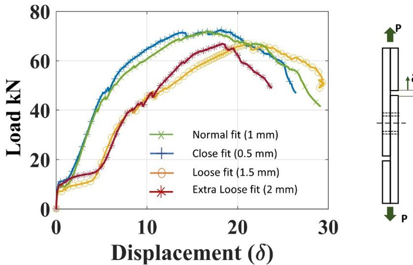
Figure 5-1: Load-displacement response of conventional bolted joint (without insert) for varying bolt-hole clearances.
