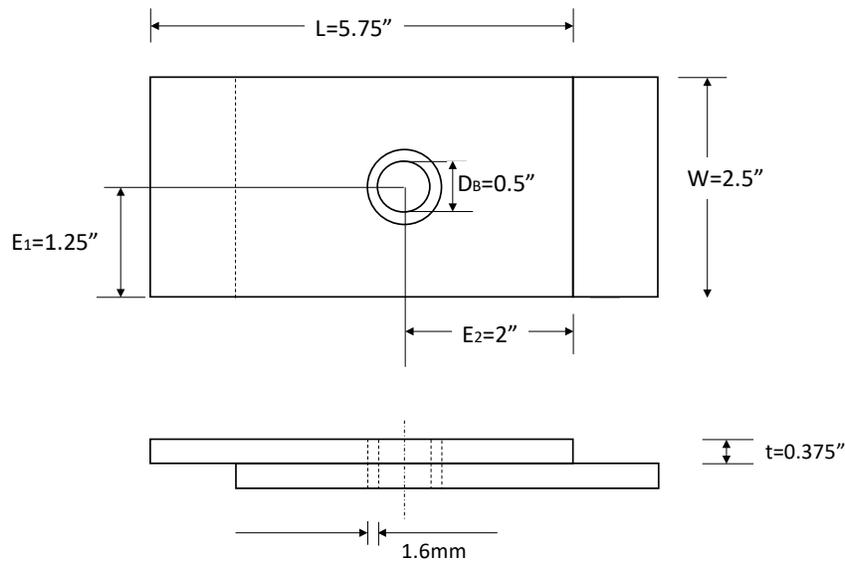
Figure 2-4: Configuration of single lap shear bolted joint specimen.
