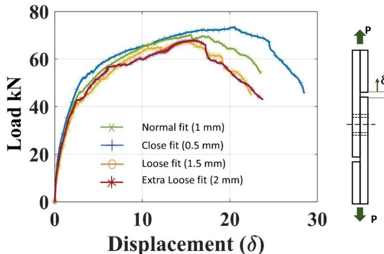
Figure 5-6: Load-displacement response of hybrid joints with aluminum-filled epoxy insert and varying bolt-hole clearances.
