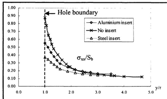
Figure 1-7: Distribution of  $\sigma_{xx}/S_b$  for different insert material along the tension plane for CFRP laminates bolted joint [24].
