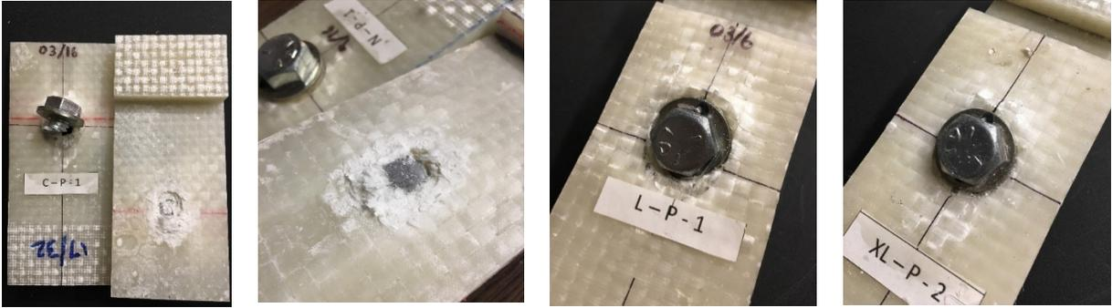
(a) Close fit (0.5mm)      (b) Normal fit (1mm),
