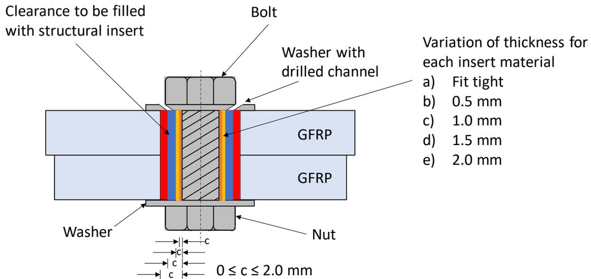
Figure 1-20. Joint configuration of hybrid fastening system for studying variations of bolt-hole clearances and insert materials.
