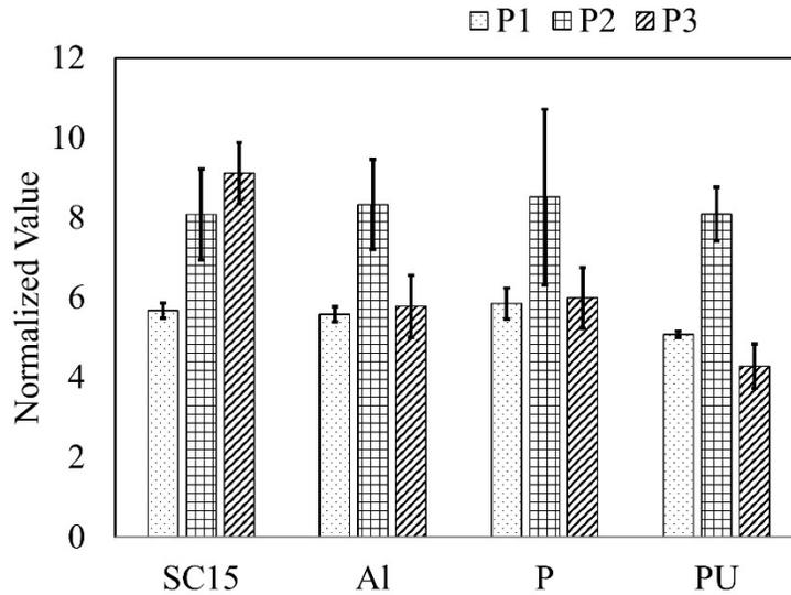
Figure 4-5: Effect of different insert material on constant clearance (1.5 mm).
