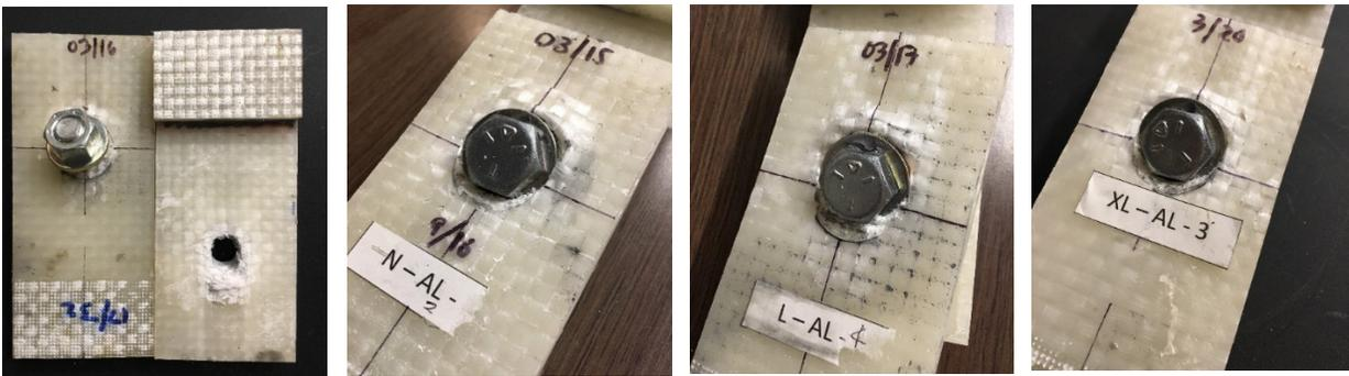
(a) Close fit (0.5mm)      (b) Normal fit (1mm),      (c) Loose fit (1.5mm)      (d) Extra loose fit (2 mm)
