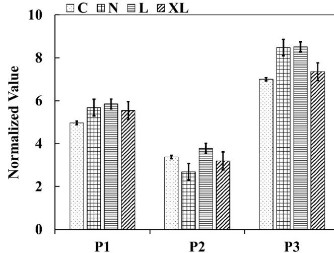
Figure 5-10: Effect of bolt-hole clearance on hybrid joints with Proset epoxy inserts
