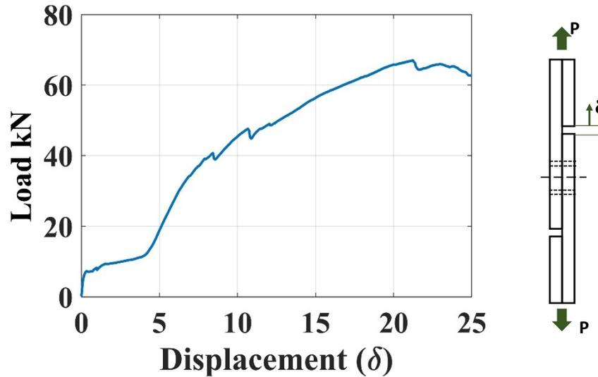
Figure 4-2: Representative Load-displacement response for conventional bolted joint (specimen L-N).
