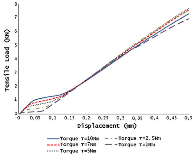
Figure 1-13: Load–displacement curves. Friction coefficient equal to 0.1. Influence of torque [27].
