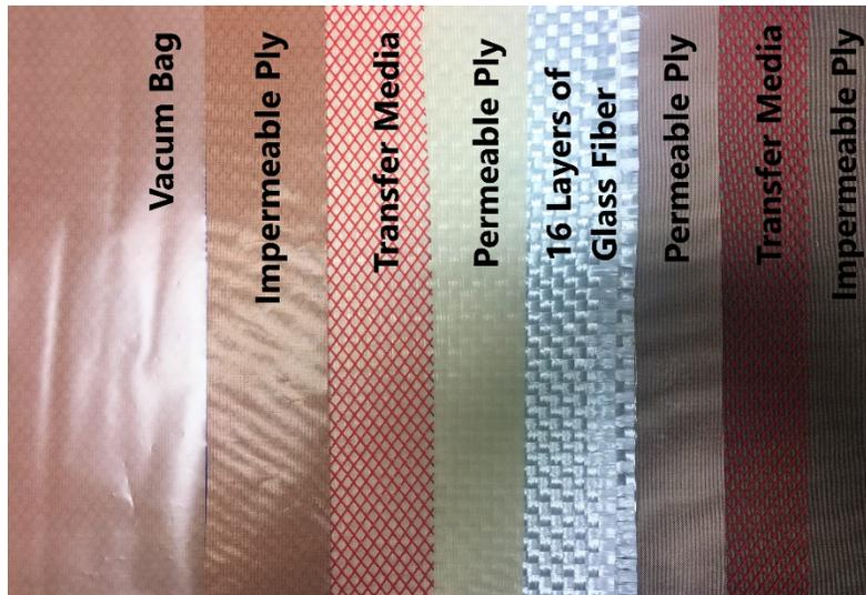
Figure 2-2: Layup for VARTM process.
