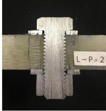
(b) Hybrid joint with PRO-SET epoxy
