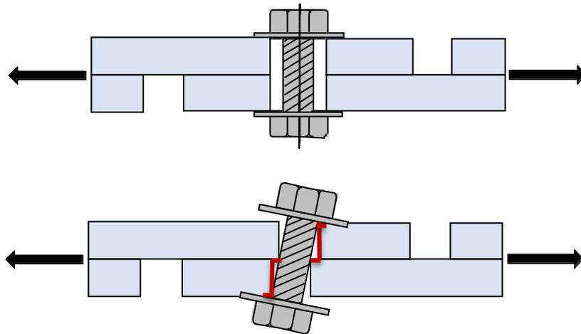
Figure 5-5: Schematic of pre- and post-slip deformation in conventional bolted joints.
