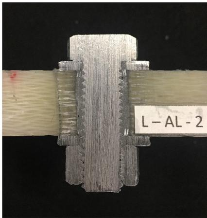
(c) Hybrid joint with aluminum liquid
