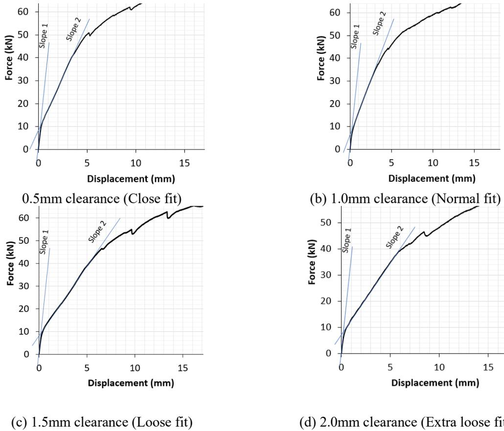
Figure 5-16: Variation in Initial stiffness of hybrid joints with Polyurethane insert as a function of bolt-hole clearance
