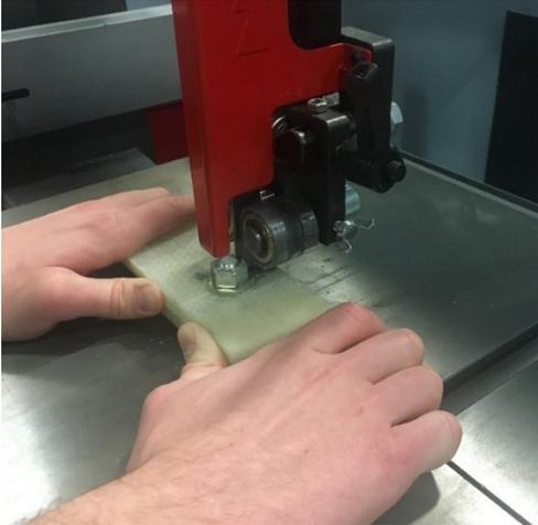
Figure 3-1: Process of cutting the cross section of bolted joints/
