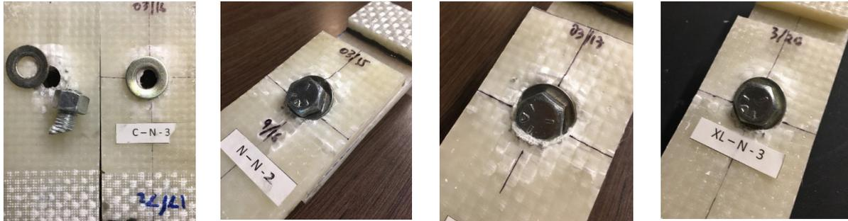
(a) Close fit (0.5mm), (b) Normal fit (1.0 mm), (c) Loose fit (1.5mm), (d) Extra loose fit (2 mm)
