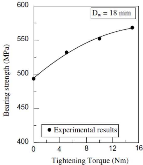
Figure 1-18: Effect of tightening torque on bearing strength of bolted joint [28].
