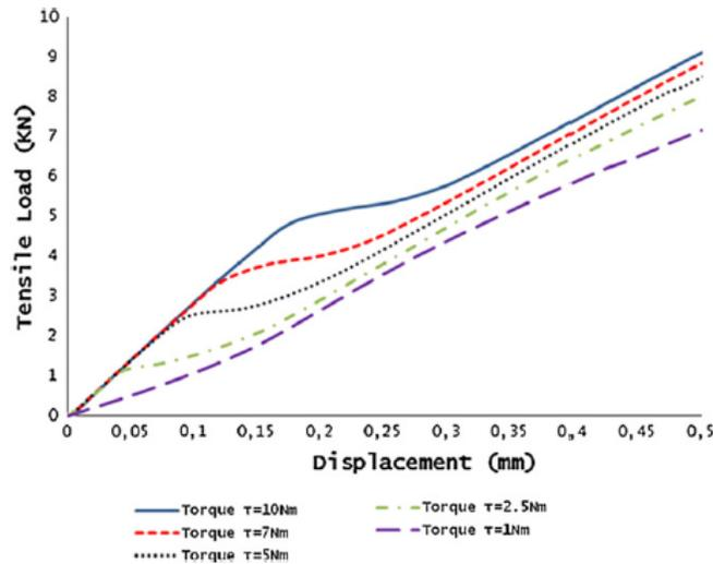
Figure 1-14: Load–displacement curves. Friction coefficient equal to 0.5. Influence of torque [27].
