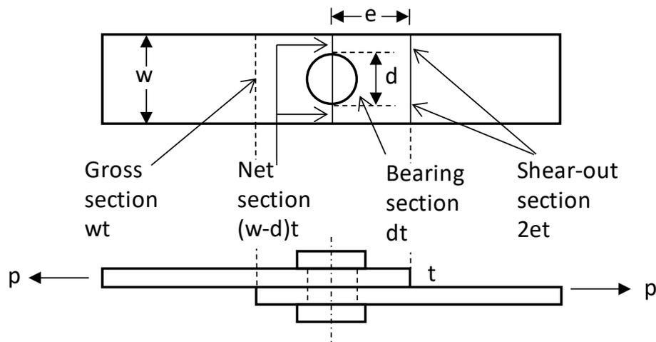
Figure 1-5: Single shear joint.
