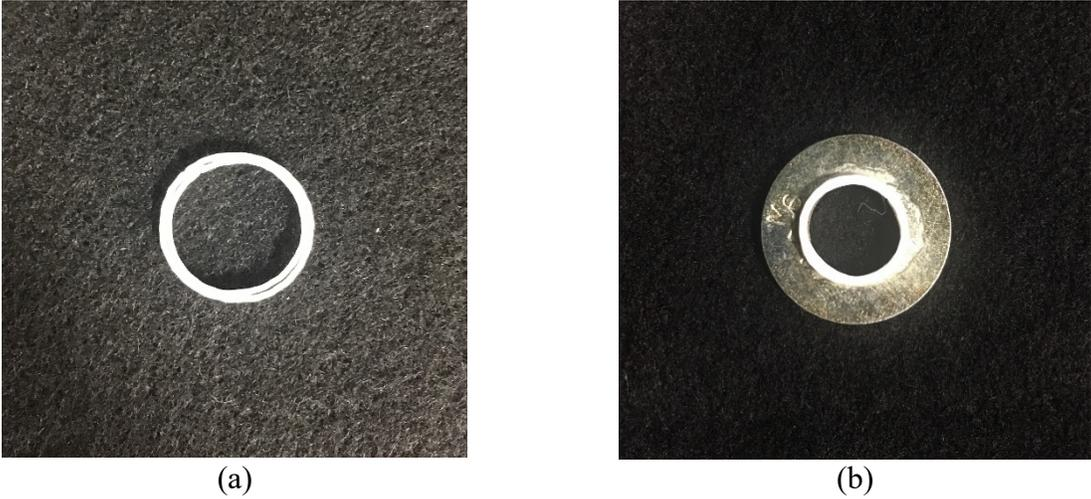
Figure 2-5: 3D printed centering washer
