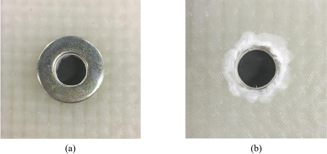
Figure 2-6: Top and bottom view of centering disc attached to washer.
