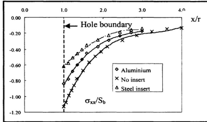
Figure 1-8: Distribution of  $\sigma_{xx}/S_b$  for different insert material along the bearing plane for CFRP laminates bolted joint [24].
