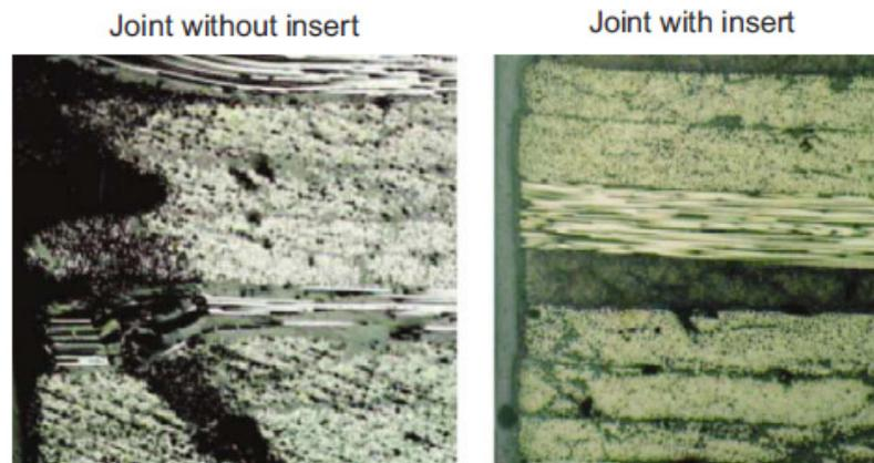
*Figure 1-12: Details of micrographs of specimens with and without inserts loaded to 7.5 kN [17].*
