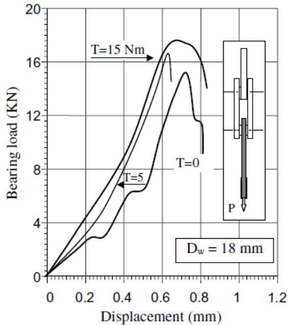
Figure 1-17: Load-displacement diagram of bolted joint with different tightening torques [28].
