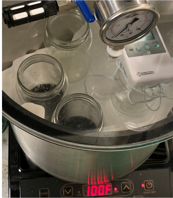
Figure 2.2: Solvent evaporation process.
