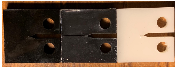
Figure 2.5: SC-15 samples, from right: baseline, 0.1wt%, then 0.5wt% of xGnP.
