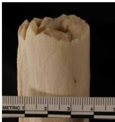
Figure 4.9: Fracture surface in a P-A impacted specimen (12-1466). The compression surface occurs on the posterior side of the bone (image left). The tension surface occurs on the anterior side of the bone (image right).
