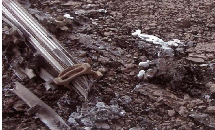
Figure 6-3. Melting of aluminum formwork supports indicating that the fire reached temperatures in excess of 650°C
