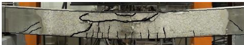
(e) Beam B1 at failure
