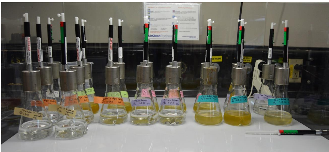
Figure 5.1 Experimental setup during passive VOC sampling of algal and bacterial samples - using SPME fibers (n=1 fiber per 250 mL flask); average exposure time ~ 2.5 hours); replicate cultures indicated by similar-colored labels.
