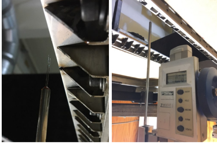
(a) Hot-wire placed 2 mm away from slit-jet nozzle (b) Hot-wire mounted on digital height gauge
