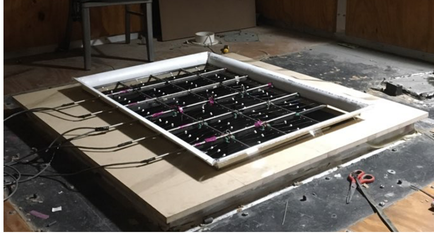
(a) TTA placed on MDF with quarter-rounds at inlet
