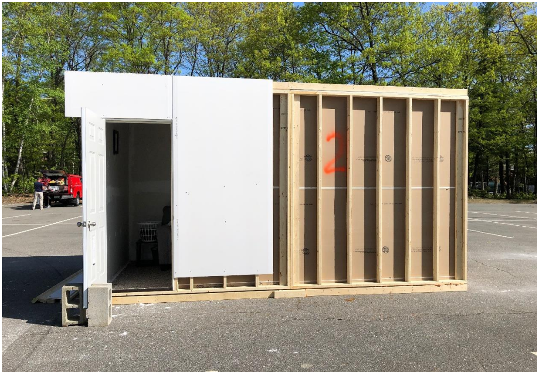
Figure A.1 Example burn cell built and used for large-scale burns
