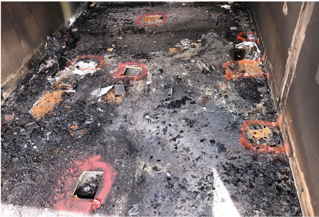
Figure A.4 Example sampling spots, circled in orange, from floor of burn cell B from which large-scale burn samples were collected
