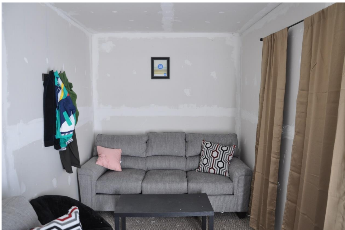
Figure A.2 Furnishings inside burn cell, including couches, curtains, coffee tables, and clothes
