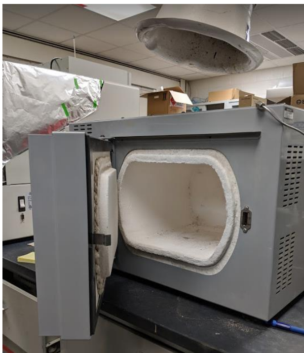
Figure 8: The outside of the F62700 Furnace used to pyrolyze the both the ferrous sulfate and the calcium-magnesium biochar
