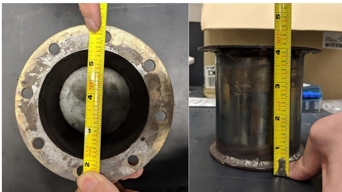
Figure 10: (Left) The rupture disc; (Right) the reactor vessel with the lid attached
