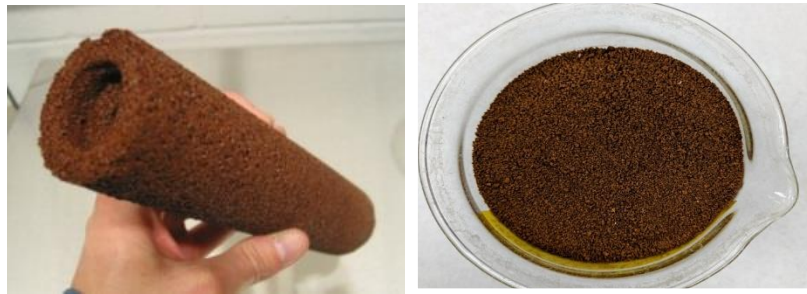
Figure 15: The PO4Sponge nano-engineered phosphorus adsorption media monolith (left) and crushed monolith granules (right) [76]
