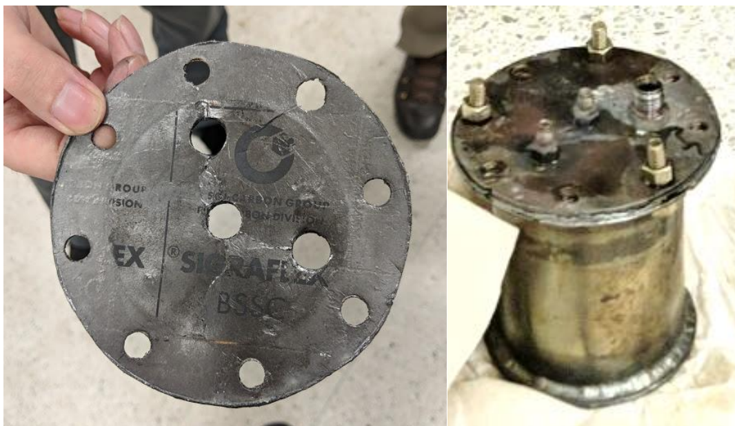
Figure 9: (Left) the snorkel fitted on top of the F62700 furnace; (Right) the interior top side of the F62700 furnace where the snorkel is located
