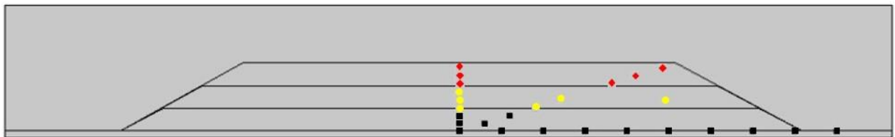
Figure 4: Schematic design: Illustrates the sugar beet pile divided into three zones, lower (■), middle (●) and upper (◆) for the 2011 season. The colored symbols illustrate the thermocouple locations as distributed in each zone.
