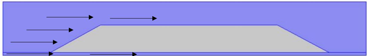
Figure 8: Schematic design: Illustrates the suggested “ventilated” sugar beet pile. The air domain is surrounding the pile from all sides. Arrows show the air direction for the model.
