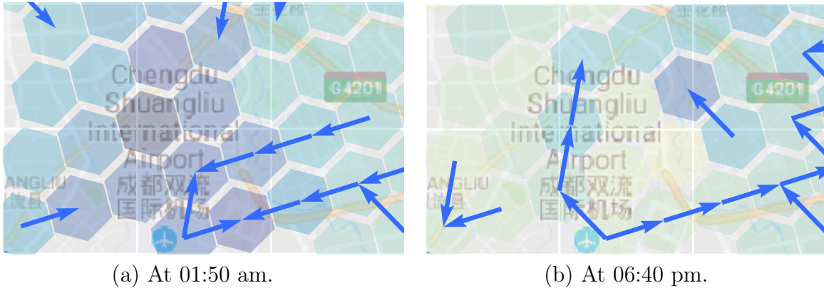
Figure 5.7: Illustration on the repositions nearby the airport at 1:50 am and 06:40 pm. The darker color denotes the higher state value and the blue arrows denote the repositions.
