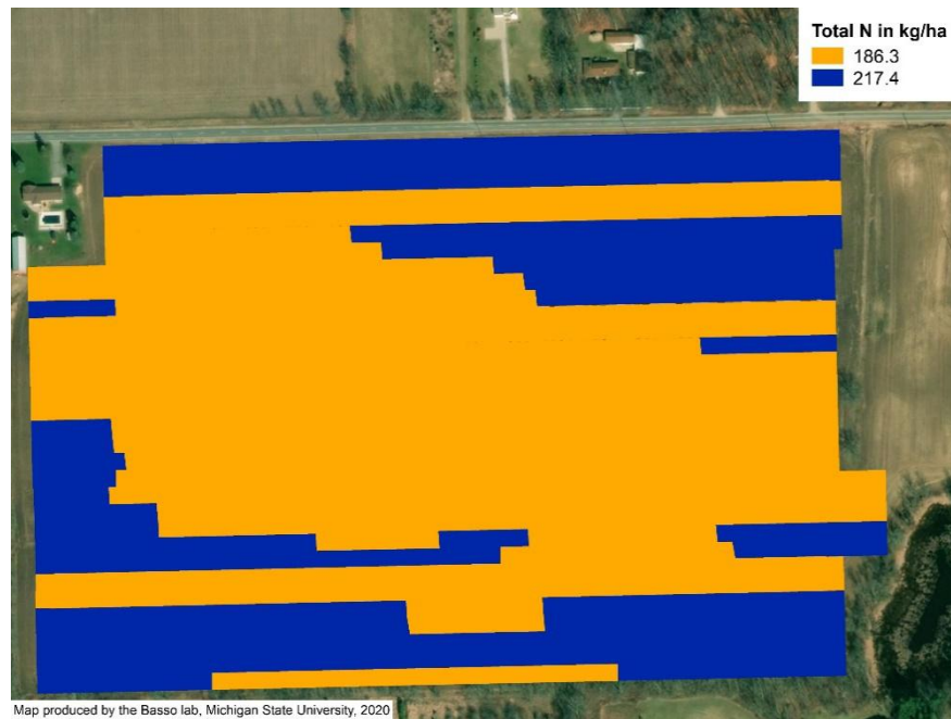
Figure 26. Nitrogen fertilizer sidedress prescription developed from remotely sensed imagery for field NC12 in 2018, created in ESRI ArcGIS.
