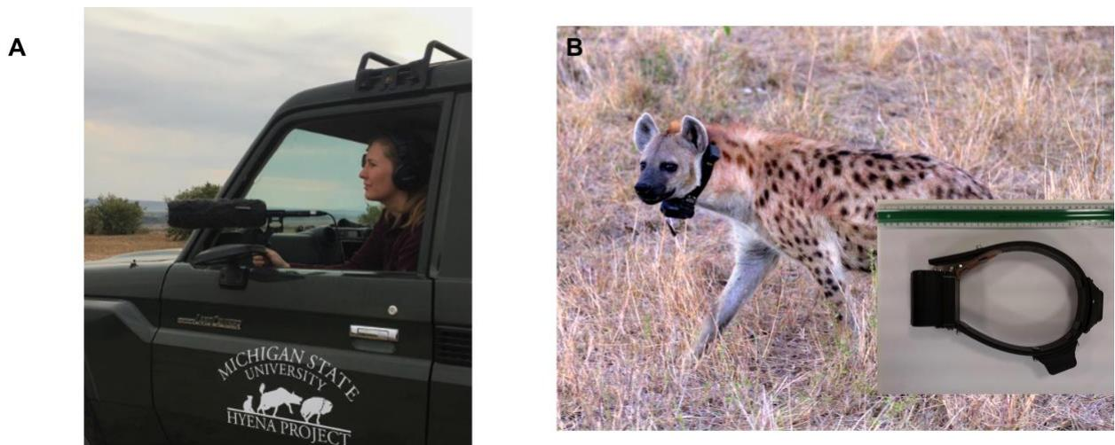
*Figure 4.2: Recording devices used: shotgun microphone handheld in the off-road vehicles we use as mobile blinds (a). and collars fitted with recording device, VHF, GPS, and accelerometers (b).*
