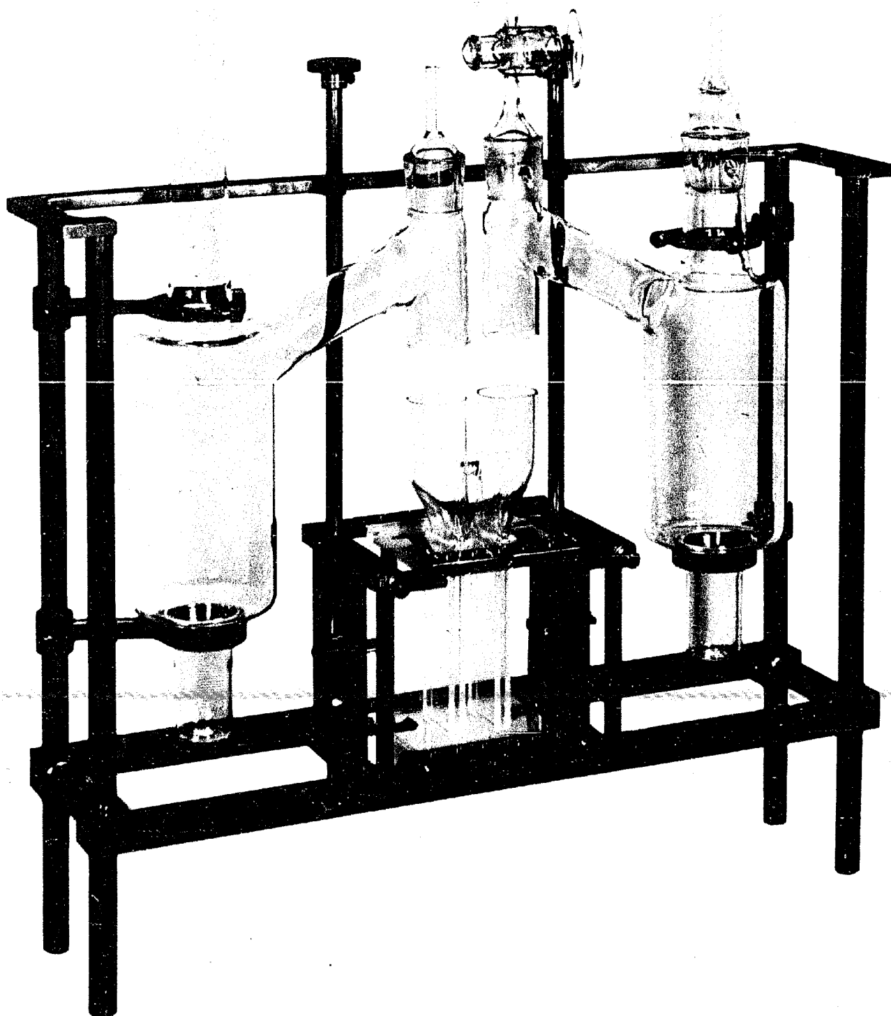
Figure 53. Electrode vessels and cell in supporting carriage. (Courtesy Klett Mfg. Co.)
