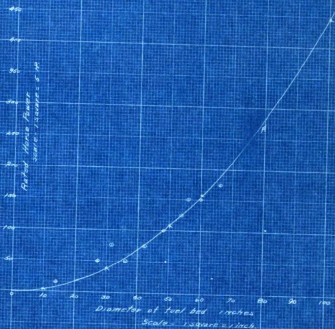
curve corresponds very closely to the points plotted from the manufacturers data and up to three hundred horse power will give results which correspond very closely with practice. For values up to about 150 H.P. the second term,  $D^5$ , can be neglected without appreciable error; in fact the equation  $H = 0.015 D^2$  is close enough for all practical purposes.
