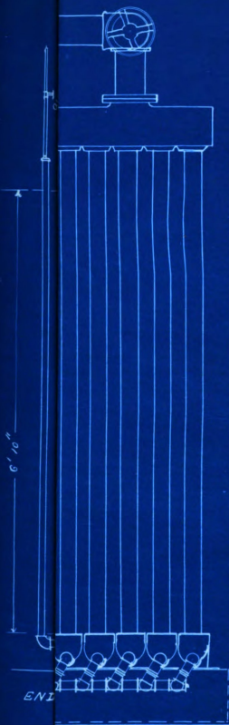
SIDE ELEVATION SHOWING FEEDERS & DRIPS
