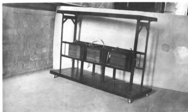
The Assembly and mounting for the Interconnected Star Transformers used with Converter R_2 .
