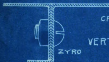
DETAILS OF JOINTS OF ZYRO AND ROSS METAL SILOS SCALE----FULL SIZE
