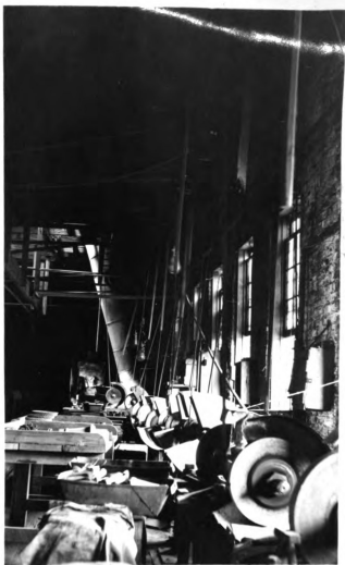
Fig. 11. The Battery of Emery Grinders showing dust hoods which maintain the suction load as long as the intakes are open. Installation of sheet iron slide valves in these and the tumbler suction pipes would have solved much of the high current cost complaint.
