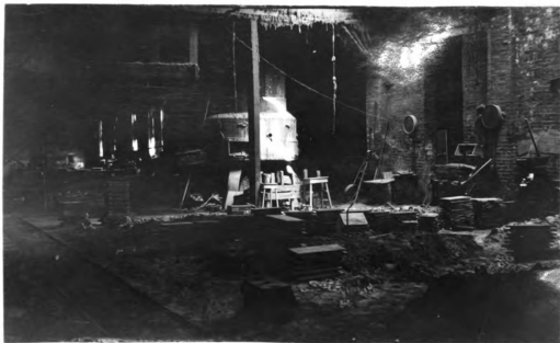
Fig. 13. Cupolas in foundry. Slag festoons can also be seen on the wires &c.
