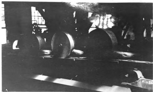
Fig. 10. Sash pulley body facing grinder showing suction connections. These castings are dropped into slots seen in the conveyor belt and passed under all three emery wheels.
