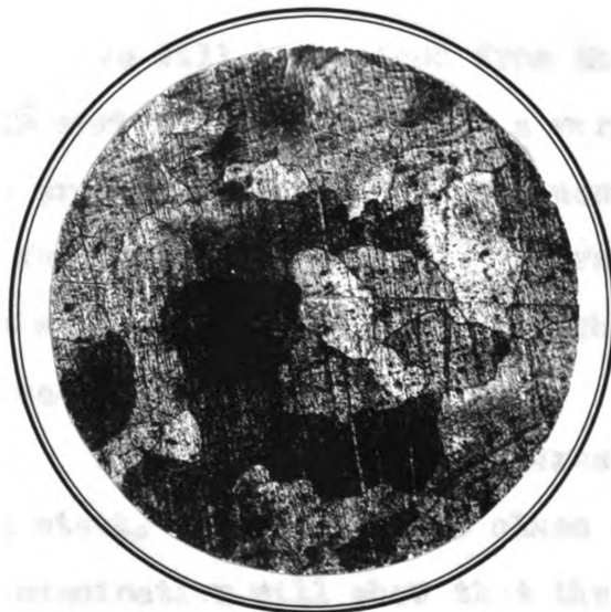
.01 Carbon Steel. Etched with \text{HNO}_3 in \text{C}_2\text{H}_5\text{OH} . Mag. 80 x Heated to 1700^\circ\text{F} and cooled in furnace 24 hrs.
