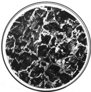
.56% Carbon Steel. Etched with \text{HNO}_3 in \text{C}_2\text{H}_5\text{OH} . Mag. 80 x Heated to 1700^\circ\text{F} and cooled in furnace 24 hrs.
