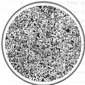
.39% Carbon Steel. Etched with \text{HNO}_3 in \text{C}_2\text{H}_5\text{OH} . Mag. 80 x Sample as received.
