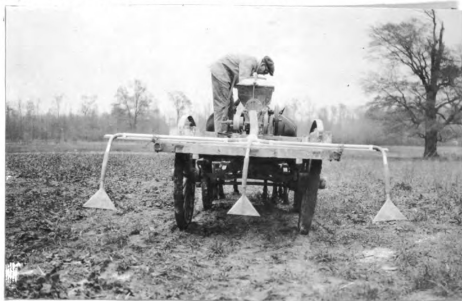
FIGURE 1. A DUSTING MACHINE IN THE FIELD SPRING, 1918. (U.S. DEPT. OF AGRICULTURE)
