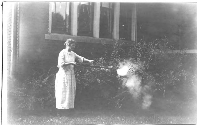
IMPROVED HANDGUN TYPE DUST BLAST GUN IN OPERATION
