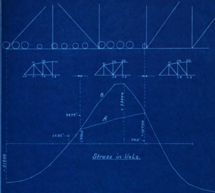
The curves marked "B" are for stiff main diagonals, those marked "A" are for counter-braced diagonals.
