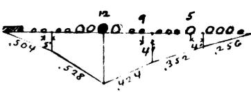
it is found that wheel 12 placed at the maximum ordinate would cause <sup>the</sup> greatest moment in a <sup>simple</sup> ~~single~~ span, the engines are headed toward the right.
