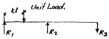
For unit load  $R_3 = -\frac{k-k^3}{4}$
