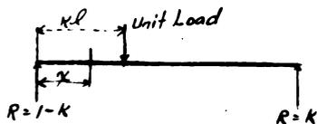
$$1. \quad EI \frac{d^2y}{dx^2} = (1-k)x \quad \text{for left segment.}$$
