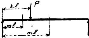
The deflection at any point of a beam loaded with any number of loads is equal to the sum of the deflections due to each load.
